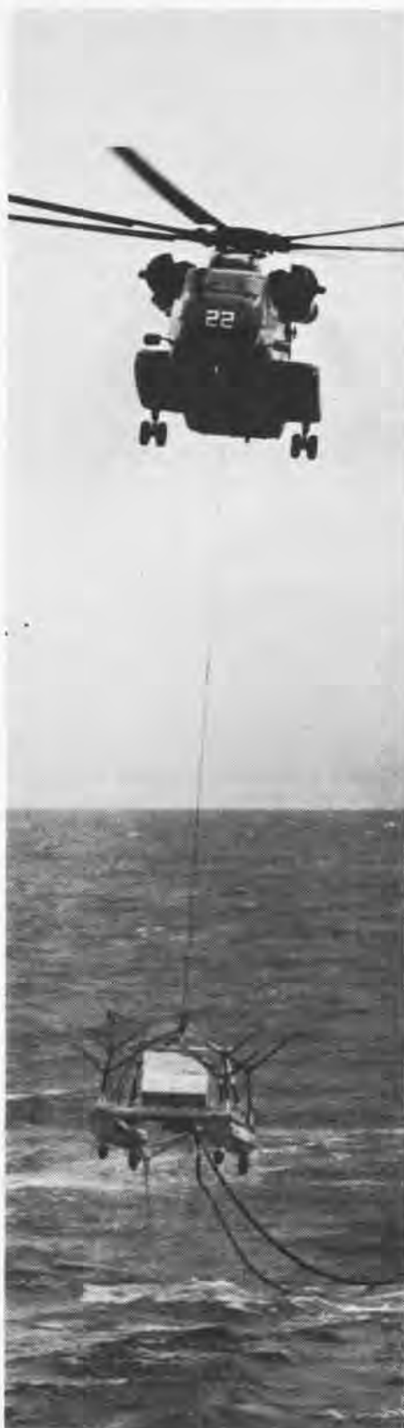
Marine CH-53A combat support helicopters were reconfigured for Navy mine sweeping operations during Operation End Sweep, the mine clearing of North Vietnamese waters.
