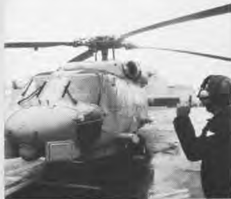
A flight line crewman signals "turn up engines" to the pilot of an HSL-43 Seahawk .
