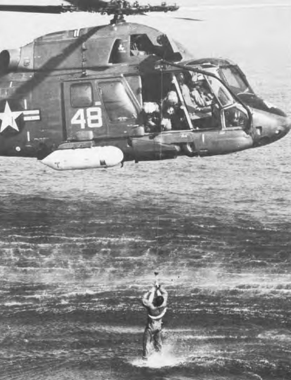
An HC-1 SH-2 Seasprite, hovering at 20 feet, uses a jet-powered hoist to pull a crewman from the water.
