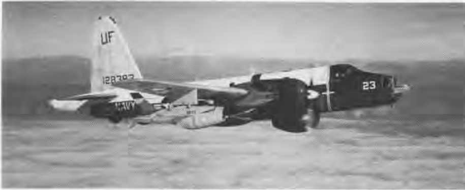
VU-3 heads out to launch two BQM-34A target drones from a squadron Neptune.
