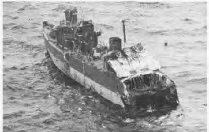
Penguin can cripple a large warship by knocking off a portion of its stern, as demonstrated in photo.
