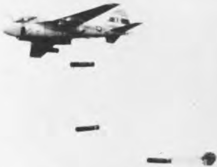
The A-6E Intruder, pictured here dropping parachute-rigged MK 50 series mines, is one of the prominent deliverers of undersea ordnance. Other chief mine-laying aerial platforms include the A-7E Corsair, S-3A/B Viking, P-3C Orion and the U.S. Air Force B-52D Stratofortress. Potential minelayers are the F/A-18 Hornet and C-130 Hercules.
