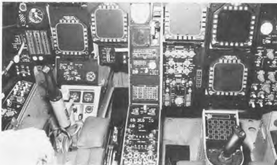
The A-6F Intruder cockpit will feature five multifunction displays which can be used to substitute each other if a malfunction occurs. The A-6F will also have a heads-up display (HUD) which will allow the pilot to monitor his speed, altitude, etc., without taking his eyes off the windscreen.
