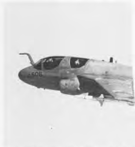
An EA-6B Prowler of VAQ-131 was the first fleet aircraft to be certified for the JT-77 turbofans.
