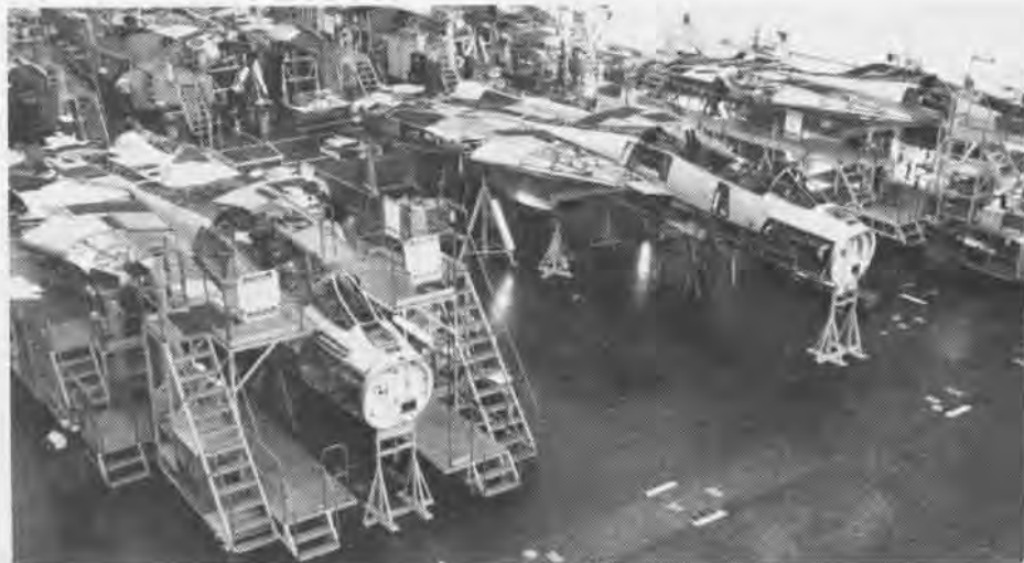
Tomcats , destined for the reserves, in remanufacture at the Grumman Calverton plant.
