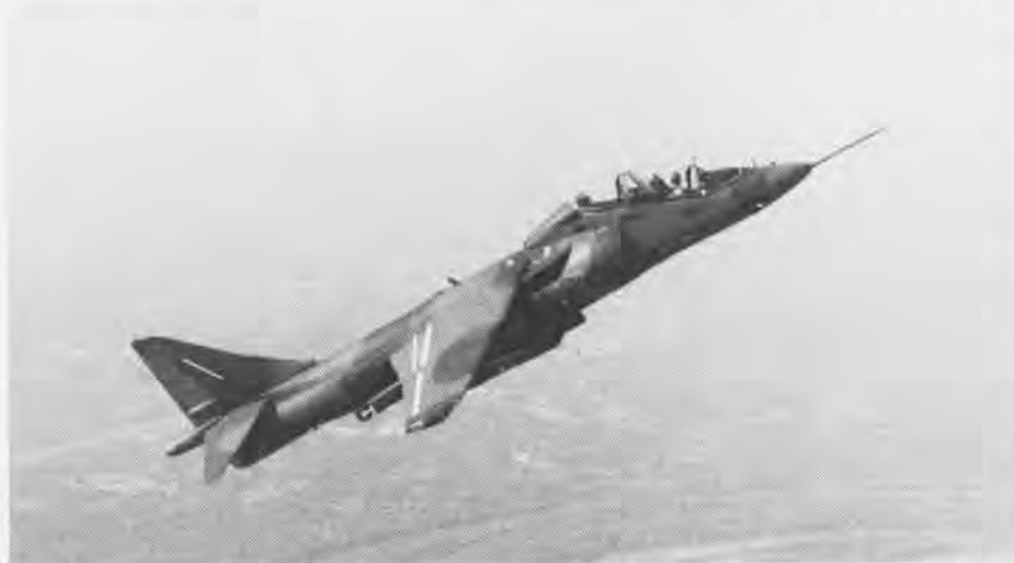
The first two-seat version of the McDonnell Douglas AV-8B Harrier II made its maiden flight over the aircraft plant in St. Louis last November. The TAV-8B will be used by the Marine Corps to train pilots in the V/STOL aircraft. The forward fuselage of the Harrier II is longer to accommodate a second cockpit and student pilots will use controls identical to those in the AV-8B. The first production TAV-8B is scheduled to arrive in the early spring at NATC Patuxent River, Md., for full-scale development testing.
