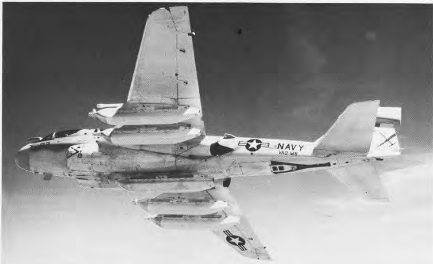
Opposite page, a Prowler of VAQ-133, NAS Whidbey Island, WA, flies near the "Deception Pass" Bridge. Above, this VAQ-129 EA-6B displays its jamming system, carried in pods — one under the fuselage and two beneath each wing.
