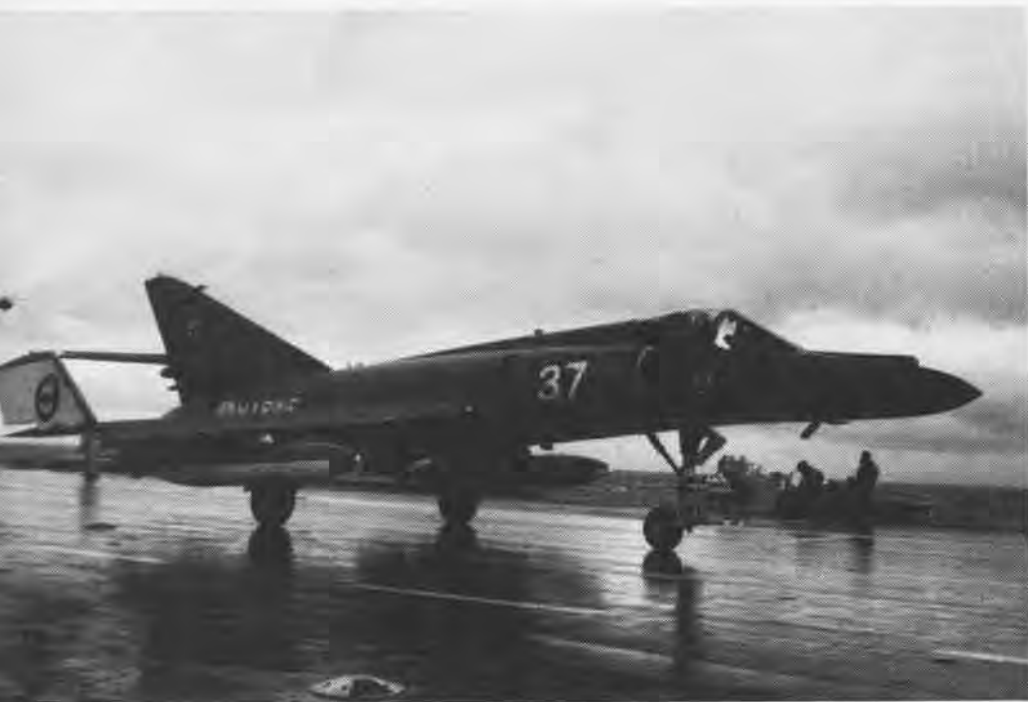
The Super Etendard is a transonic, single-seat strike-fighter flown from Clemenceau-class aircraft carriers.
