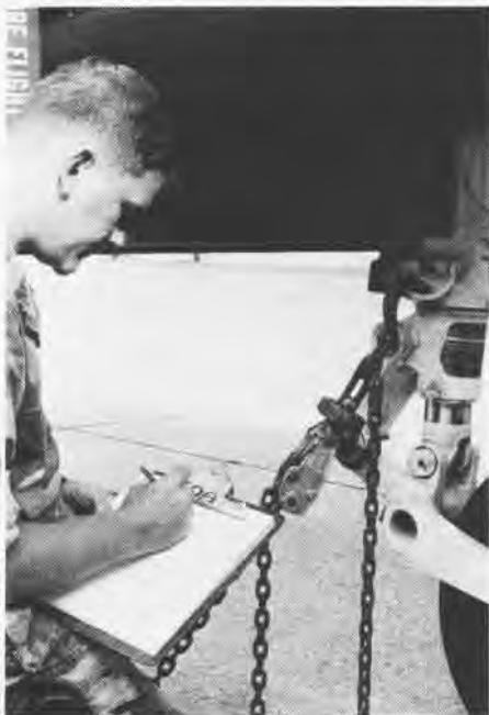
SSgt. R. W. Kitchens, air frames inspector, checks for corrosion on an OV-10 Bronco from VMO-2.
