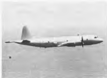
A P-3 from VP-46 sports a low-visibility paint scheme. This Orion is configured with an ALQ-157 infrared survivability and vulnerability enhancement device.
