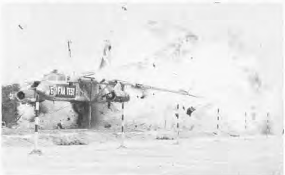
NAEC's Test Department intentionally crashes an RB-66 aircraft on one of its five high-speed test tracks during a Spring 1983 test conducted for the Federal Aviation Administration. The test was designed to evaluate a jet fuel additive which prevents misting of the fuel to reduce the potential of post-crash fires and fatalities.
