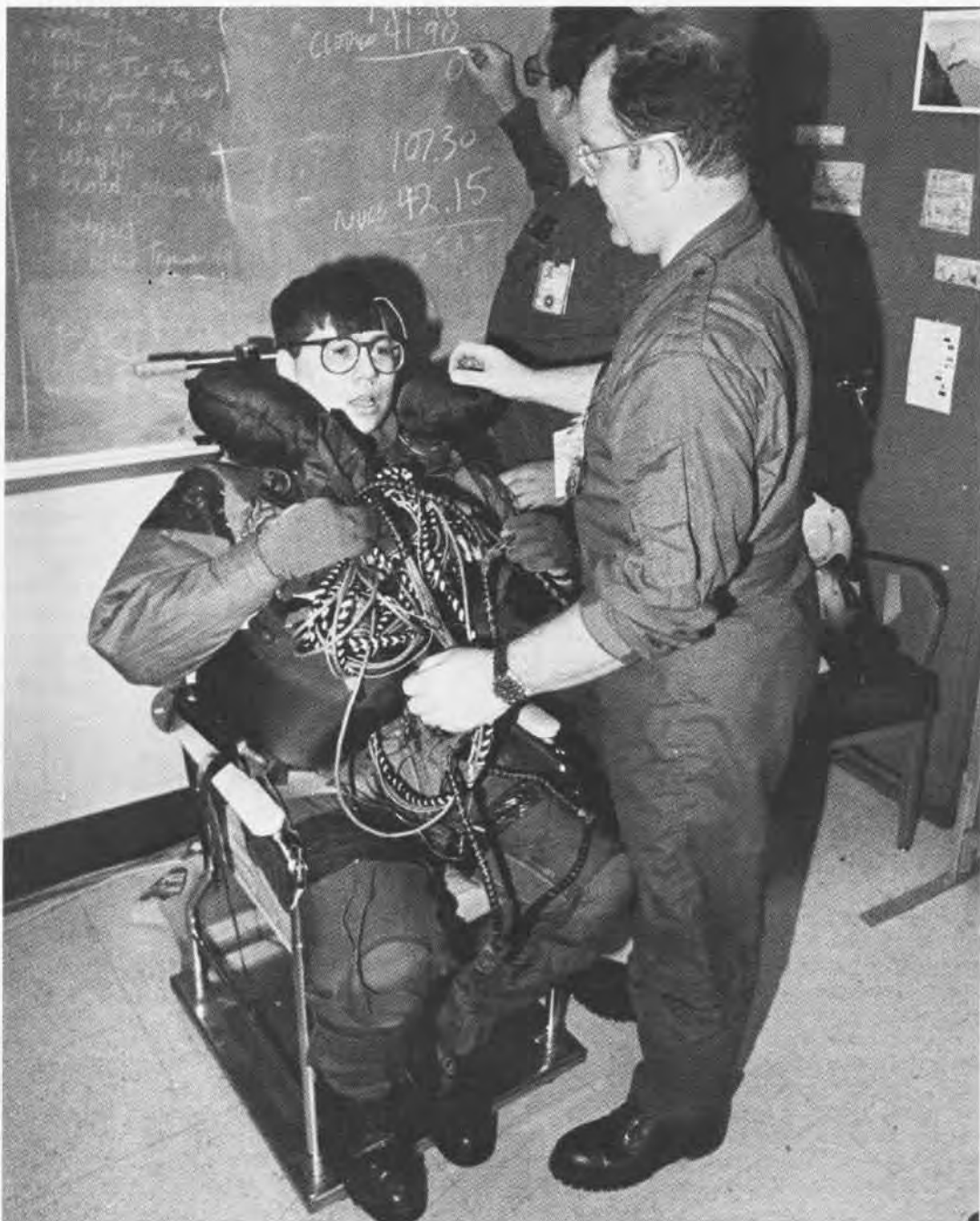
HM2 Elvin Santiago prepares to spend a couple of hours in frigid temperatures to help test the CWU-62/P antiexposure suit. PR1 Robert Elliott helps him suit up.
