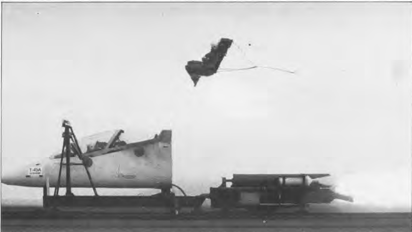
A three-point drogue harness increases the seat's stability by keeping the seat facing into the airstream.
