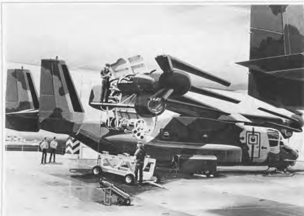
The Osprey has a unique folding capability which gives it less restricted shipboard ops.
