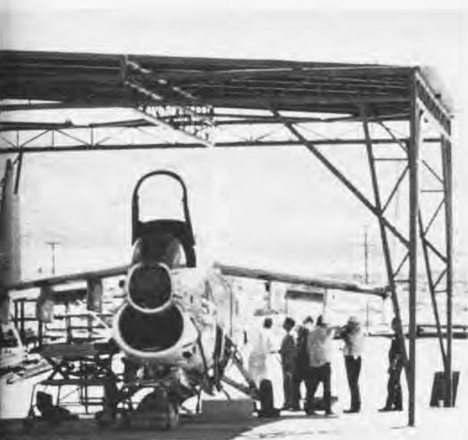
Far left, students assess damage and perform repair on aircraft structures that have been ballistically impacted. This provides invaluable experience in tracing projectile penetration through the airframe and components. Left, salvaged jets serve as training platforms for battle damage repair training. Above, practicing battle damage repair using special tools from the ABDR kit provides realistic experience to prepare fleet personnel for wartime repair practices.
