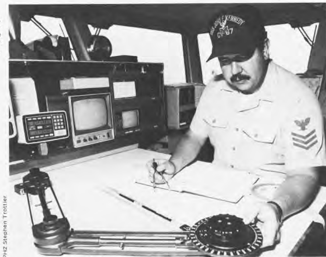
A quartermaster aboard John F. Kennedy (CV-67) plots the carrier's position at sea with the aid of the NAVSTAR GPS console and a sextant.
