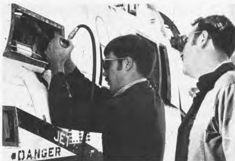
Far left, students assess damage and perform repair on aircraft structures that have been ballistically impacted. This provides invaluable experience in tracing projectile penetration through the airframe and components. Left, salvaged jets serve as training platforms for battle damage repair training. Above, practicing battle damage repair using special tools from the ABDR kit provides realistic experience to prepare fleet personnel for wartime repair practices.
