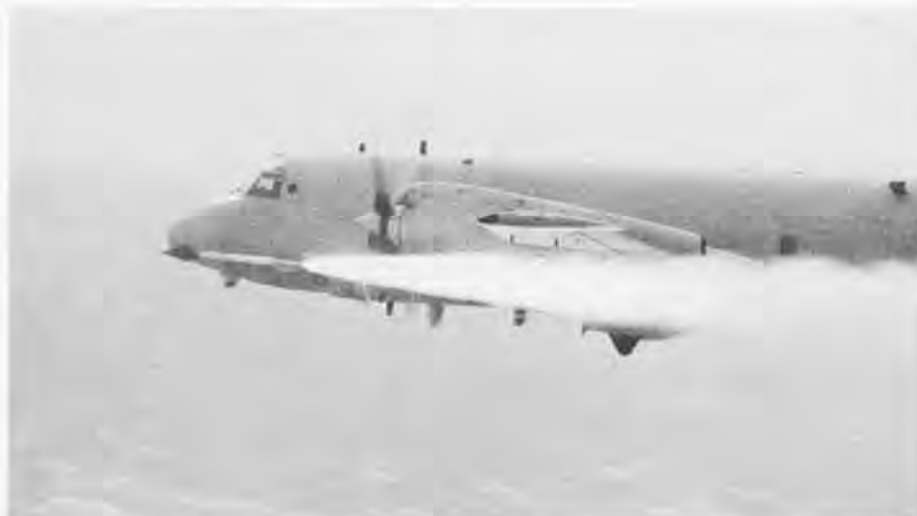
A P-3 Orion from NATC Patuxent River, Md., launches an AIM-9 Sidewinder during tests of the air-to-air missile as a defense weapon for antisubmarine warfare patrol aircraft.
