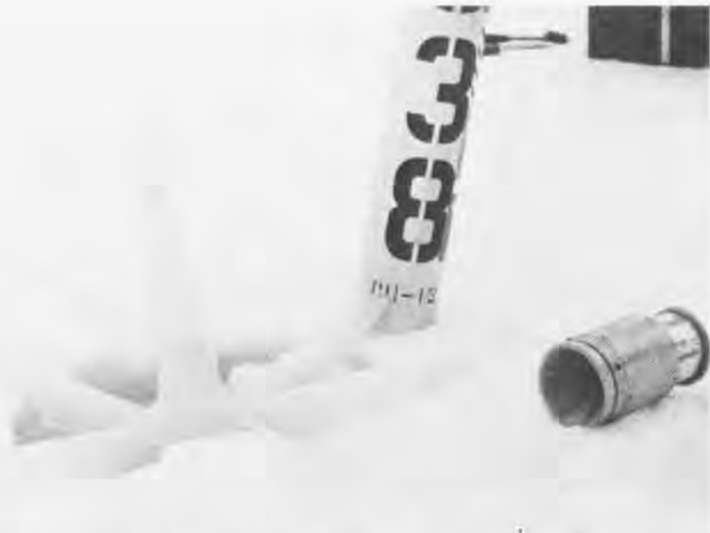
Thermal buoys were tested during ICEX-1-89. Producing their own heat, they melt through the ice.
