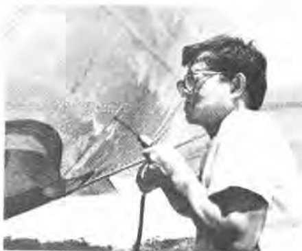
FAWPRA Filipino National employee Israel Mangibin removes a cracked cargo door fitting from a VMFA-152 KC-130F.
