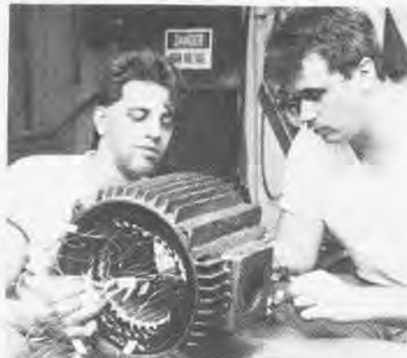
EM3 Dominic C. Rotondo and EM3 William Gallagher rewind an electric motor as part of their duties with Enterprise's Engineering Department.
