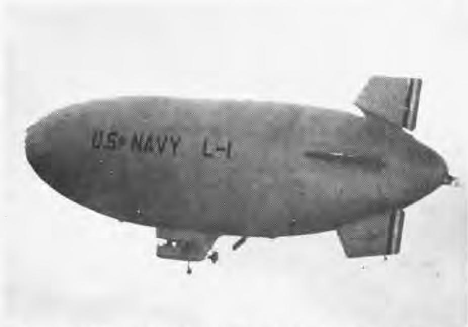
The Goodyear L-1 nonrigid airship was ordered in 1937 as a trainer for follow-on airships.
