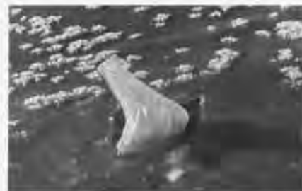
A sonobuoy that has surfaced through the ice (April 1985, Central Arctic)
