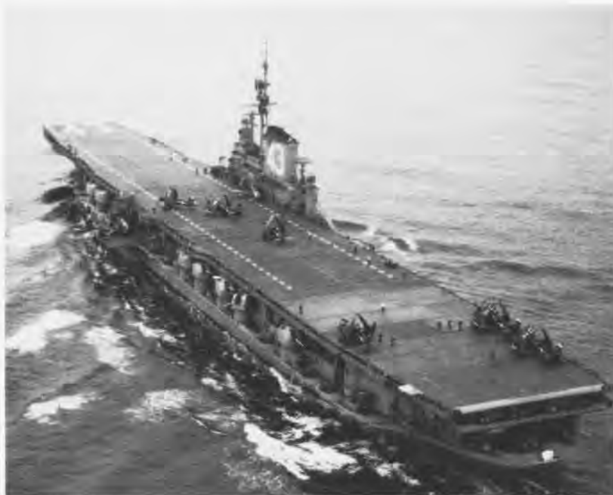
Straight-decked Coral Sea as she looked in 1947 shortly after commissioning, complete with 14 5-inch guns.
