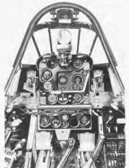
SBD-6 pilot's instrument panel with Mk 8 illuminated gun sight and Browning .50-caliber machine guns installed. Chart board between two sections of instrument panel is partly withdrawn. Note the gun charging handles and canvas pouch tied around the lower rear of the guns to absorb oil and prevent it from dripping on the pilot's leg.
