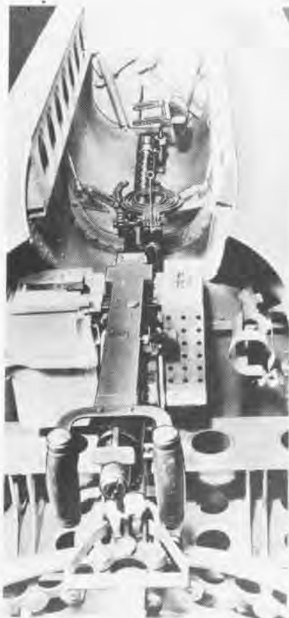
SBD-1 original single .30-caliber free gun installation. Note 100-round magazine on gun and holder for six more.
