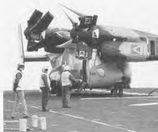
The complex wing and rotor-folding arrangement of the MV-22A Osprey is evident in this view taken during shipboard compatibility trials aboard Wasp (LHD-1).
