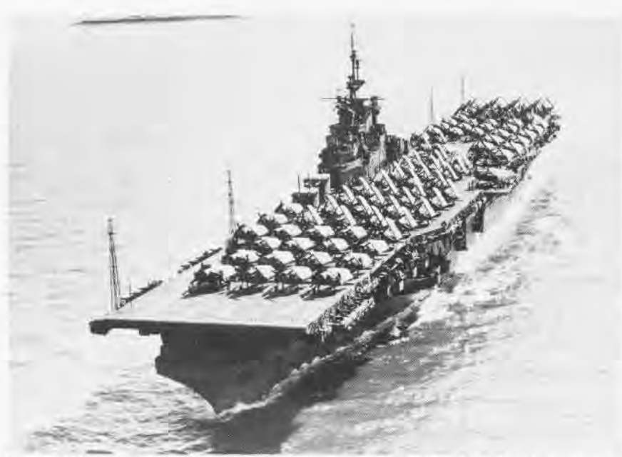
Boxer (CV-21) with her 1945-model air group. Most of the flight deck is taken up by the Hellcats and Corsairs of her two 36-plane VF squadrons. Smaller squadrons of Avengers and Helldivers are spotted astern. A typical late-war task group – 3 CVs and 2 CVLs – could put nearly 400 planes into the air, carrying over 214 tons of bombs and 2,000 five-inch rockets, to strike targets at ranges of 250 miles or more.
