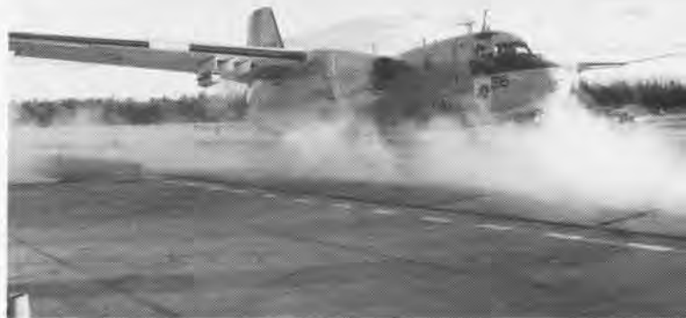
A Brazilian Air Force S-2 Tracker antisubmarine aircraft underwent catapult launch and arrested recovery trials late last year at the Naval Air Engineering Center, Lakehurst, N.J., after being reengined with turboprops in Canada.
