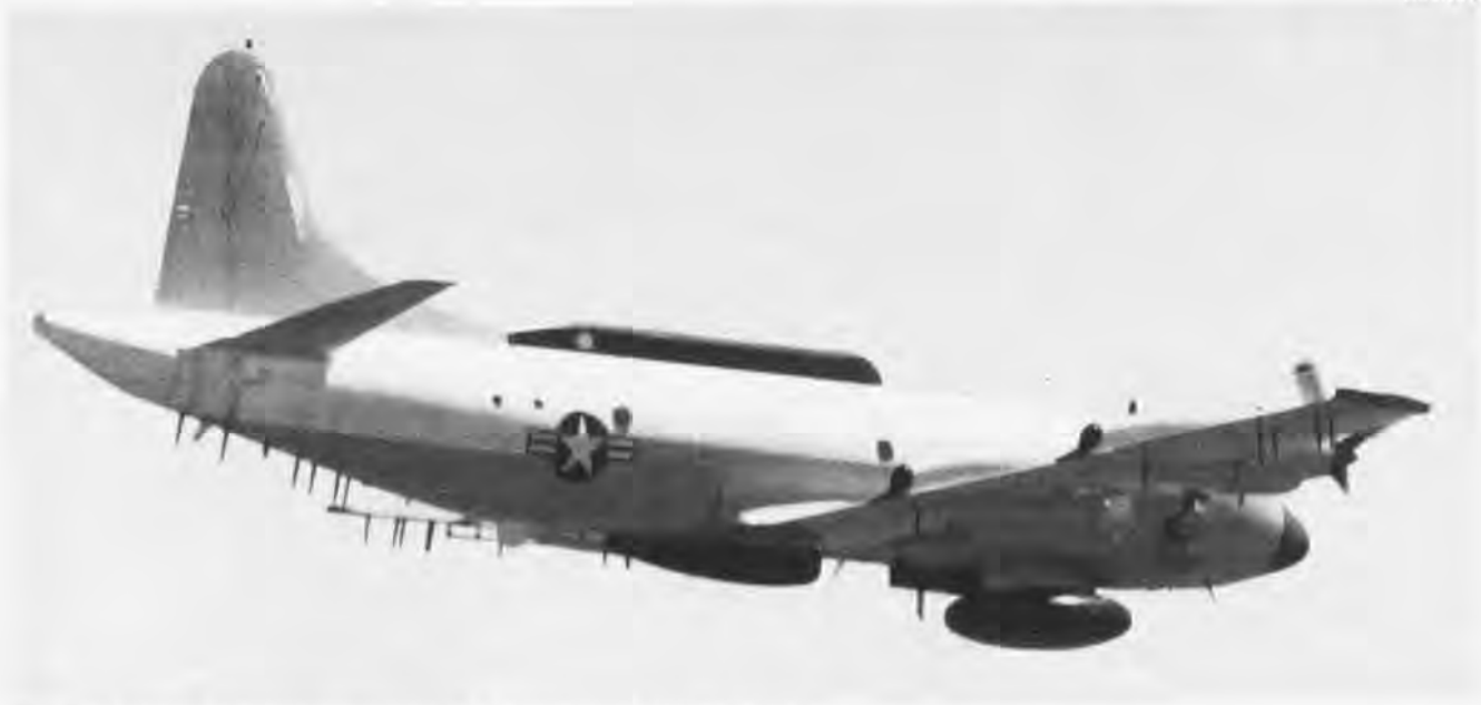
The EP-3E Aries II is replacing aging EP-3 Aries I aircraft in VQs 1 and 2.
