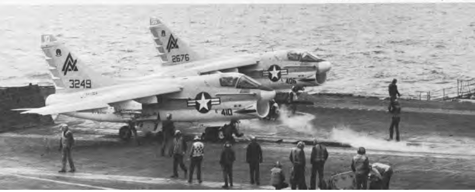
A-7As from VA-304 taxi onto Ranger 's waist catapults in preparation for launch.
