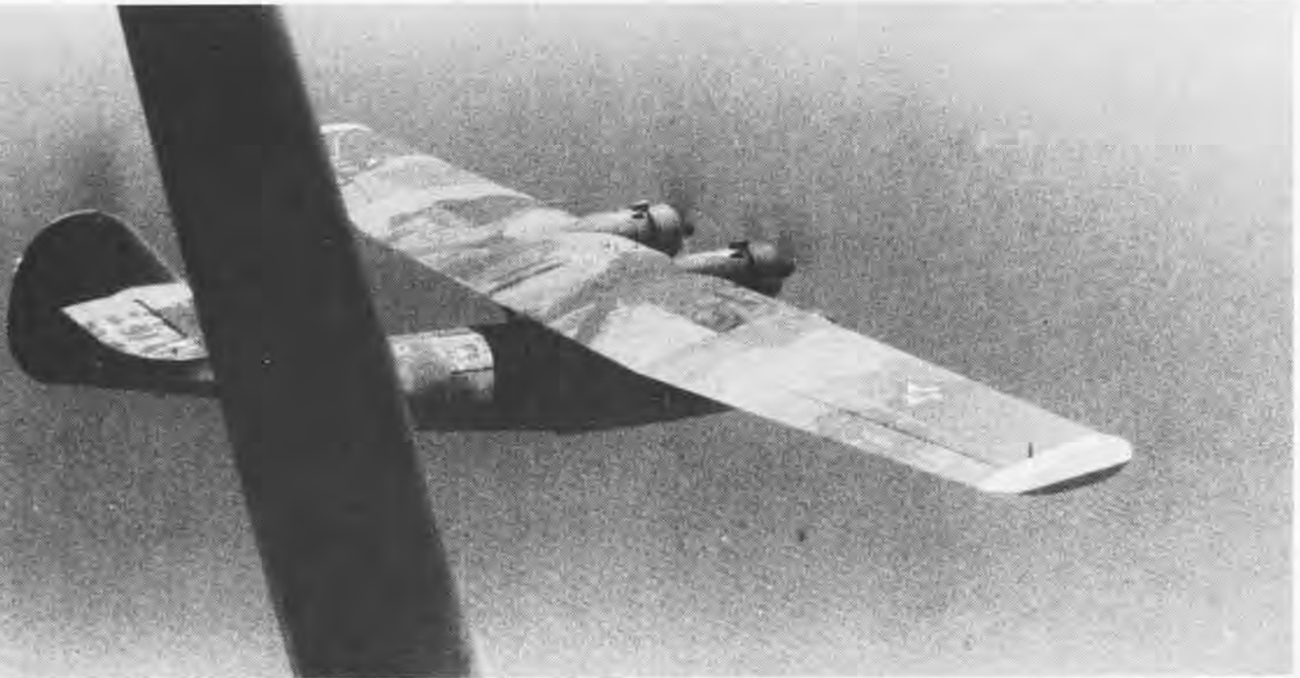
Asiatic Fleet camouflage on a PatWing-10 PBY-4. The lack of waist blisters and the older style rudder identify this as a "Dash 4" but the locally prepared multitone scheme, thought to be shades of blue and gray, conceals nearly all the former markings.
