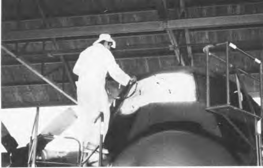
Jerry Plunkett, an AMARC employee, applying the last layer of white Kool Kote.
