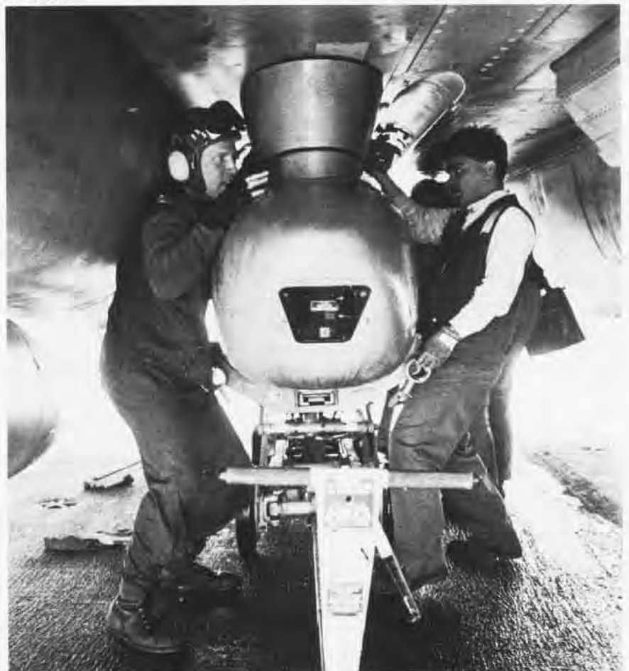
VF-84 crewmen PH3 Pat Ross and PH3 Aerillo Ayuso prepare a Tactical Aerial Reconnaissance Pod System on an F-14A for a photoreconnaissance mission over Iraq during Operation Provide Comfort.
