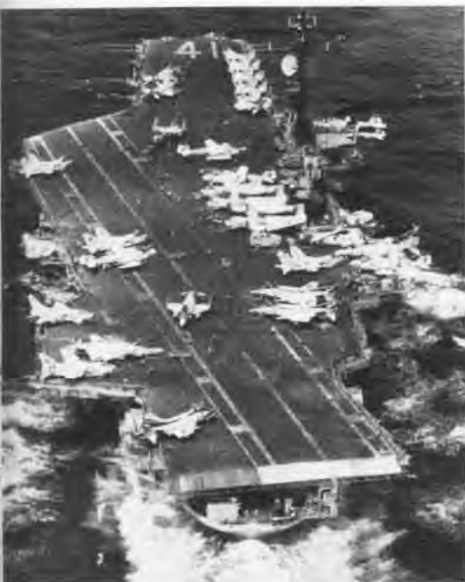
Midway , November 30, 1974, underway in WestPac, showing clearly the layout of the flight deck with the two starboard side deck-edge elevators. KN-22932
