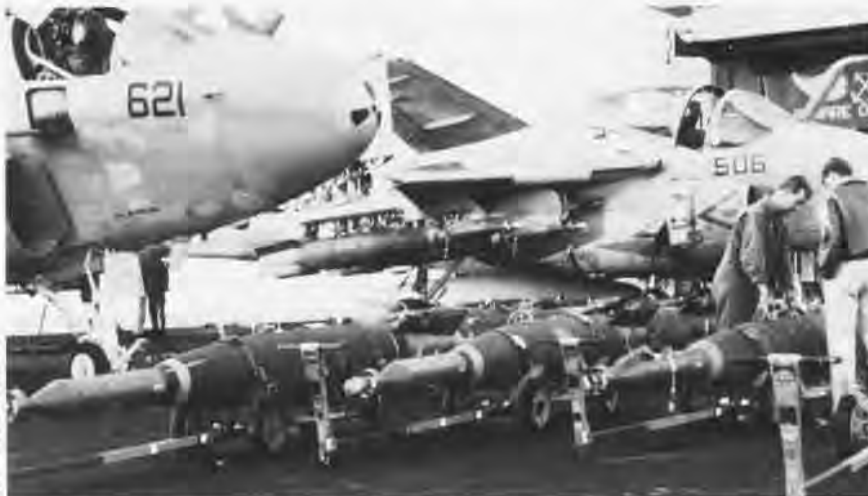
GBU-10E/B Paveway II laser-guided bombs are prepared for war on the deck of John F. Kennedy (CV-67) the day before Desert Storm began.
