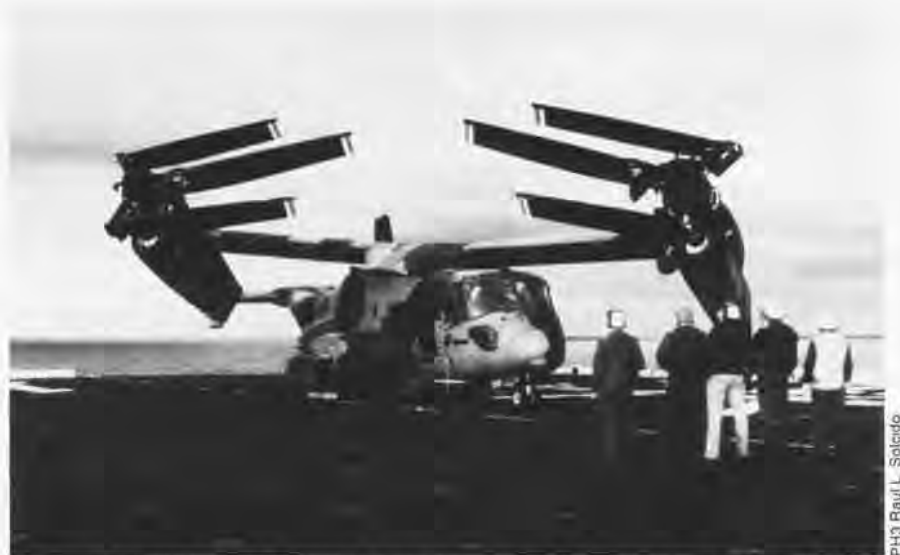
Sea compatibility trials of the V-22A, seen here folding its rotors aboard Wasp (LHD-1), were conducted during December 1991.
