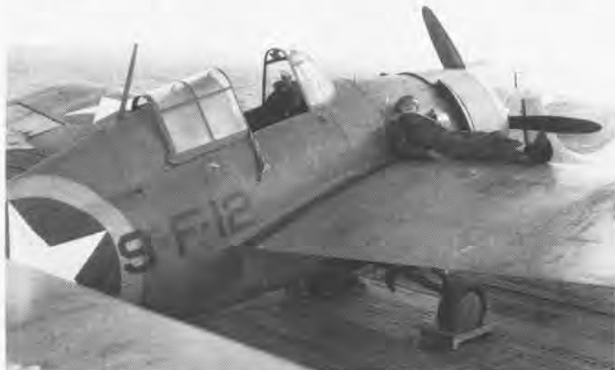
A plane captain relaxes on the wing of 9-F-12, a Wildcat of VF-9. Note the strap from the pilot's harness spread over the cockpit sill.
