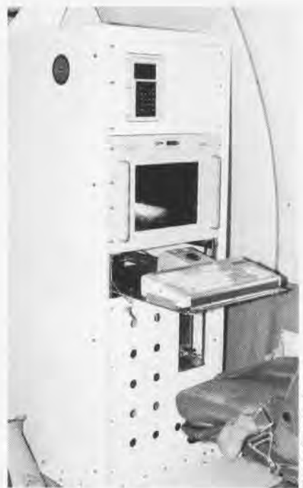
The Advanced Tactical Workstation installed in the aft fuselage of the Outlaw Hunter P-3C.
