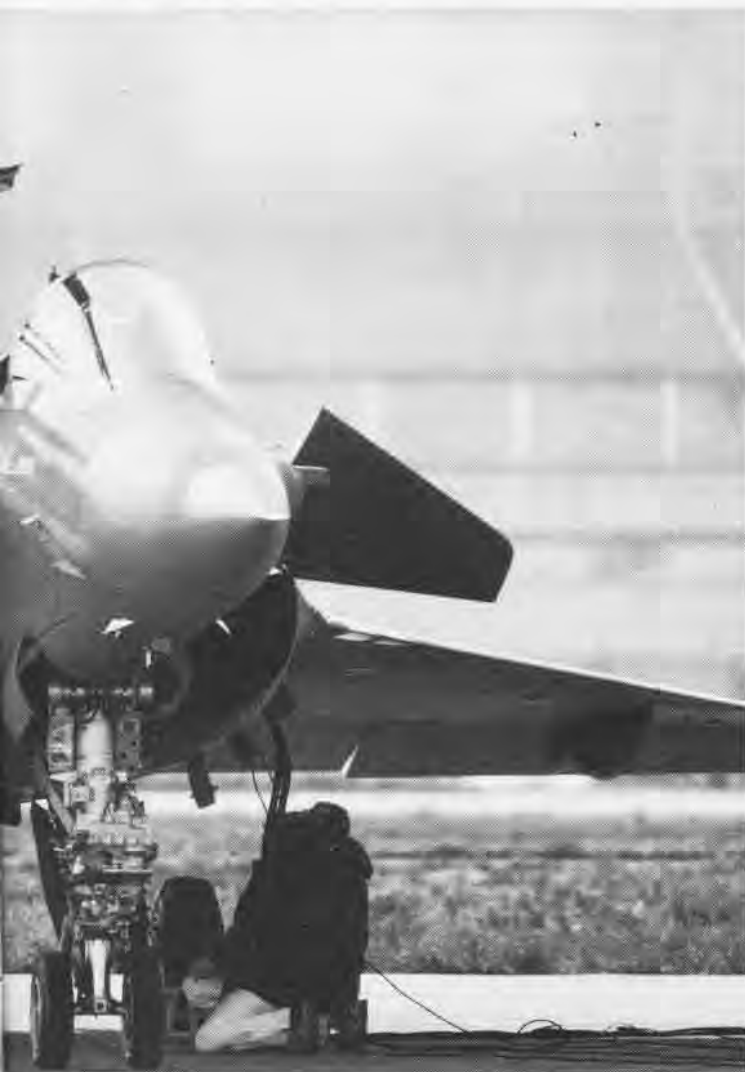
Frances's new naval fighter, the Rafale M01 , underwent an extensive set of aircraft platform interface tests this past summer at NAWC AD Lakehurst, N.J. The tests included catapult launches, arrested landings, and jet blast deflector tests.
