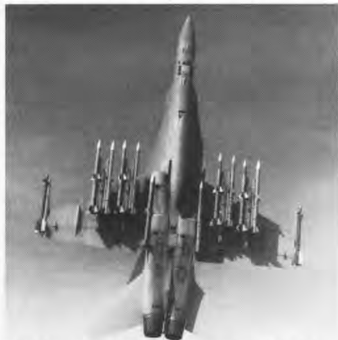
Twelve stingers on this Hornet — An FA-18C assigned to VX-4, NAWS Point Mugu, Calif., displays air-to-air weaponry consisting of 10 AIM-120 AAMRAM missiles (under wing and on fuselage stations) and two wingtip-mounted AIM-9 Sidewinders.
