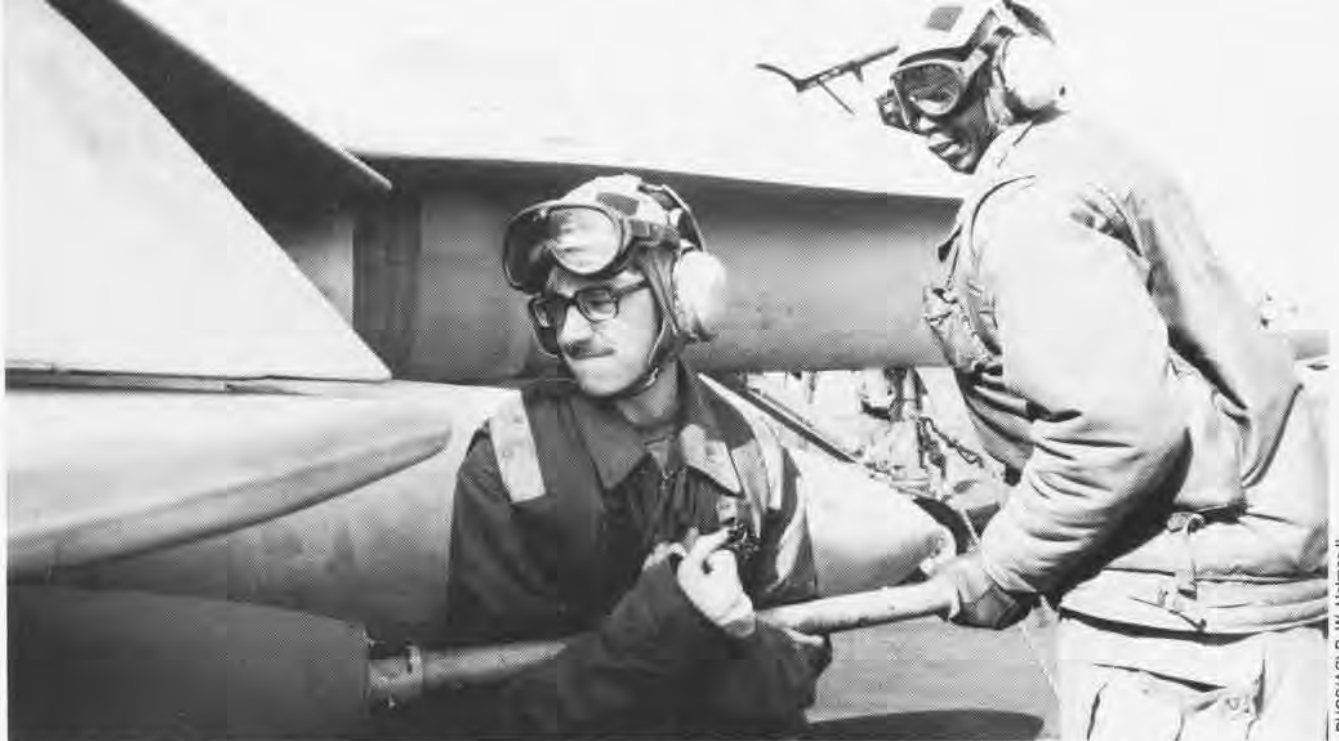
AOs of the VFA-105 Gunslingers load a MK-37 500-pound practice bomb onto the wing of an FA-18 Hornet onboard Kennedy (CV 67).
