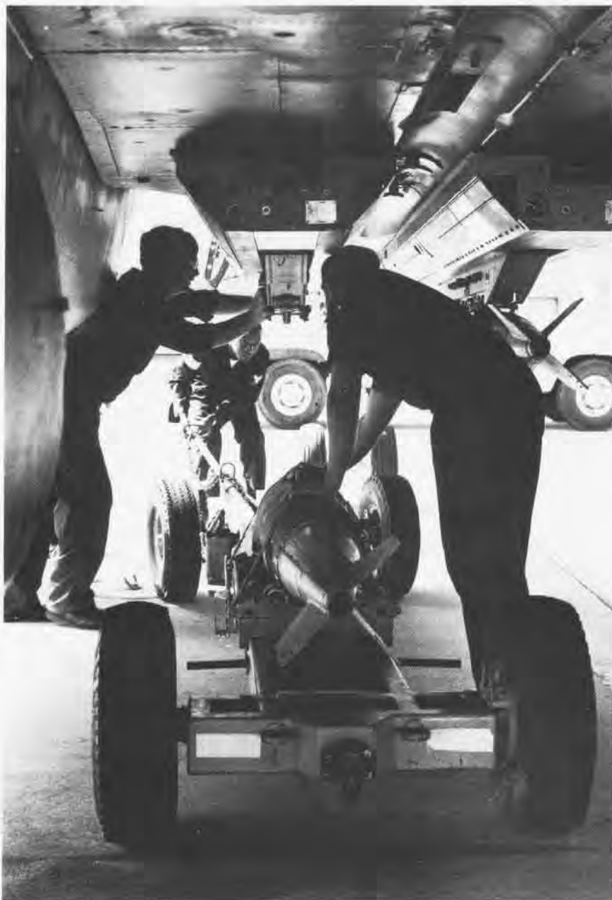
Teamwork, attention to detail, and double checking every procedure are critical to the safety of the personnel of Strike Division, NAWC AD Patuxent River, as they load a MK-82 bomb onto an F-14A.
