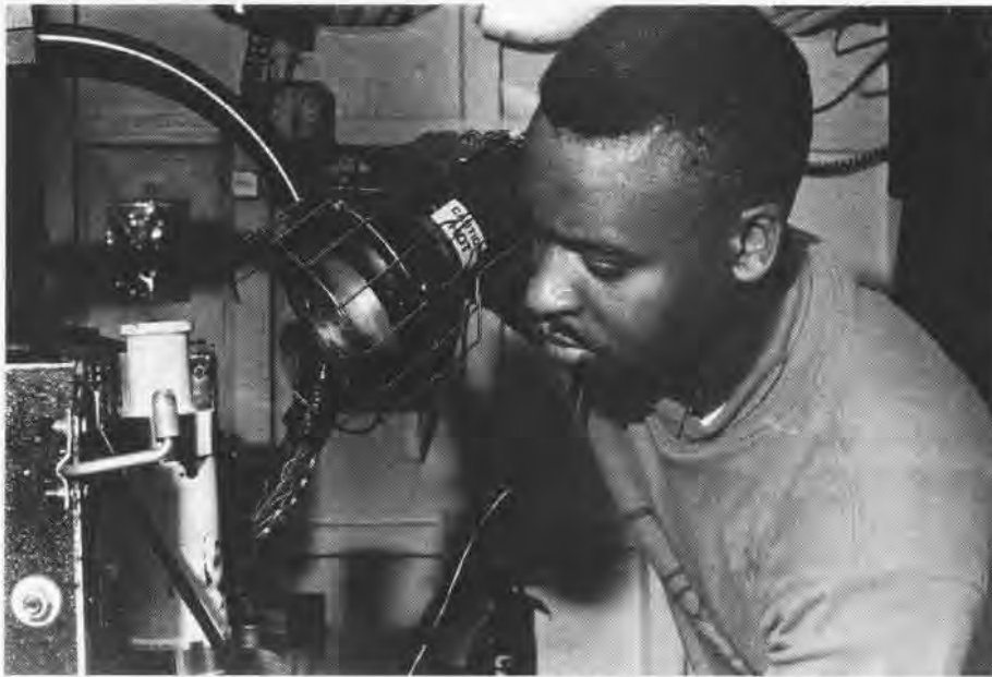
During a magnetic particle inspection, AMS2(AW) Vernon Brown checks for cracks and defects in a hydraulic cylinder. Brown is assigned to the AIMD onboard Theodore Roosevelt.
