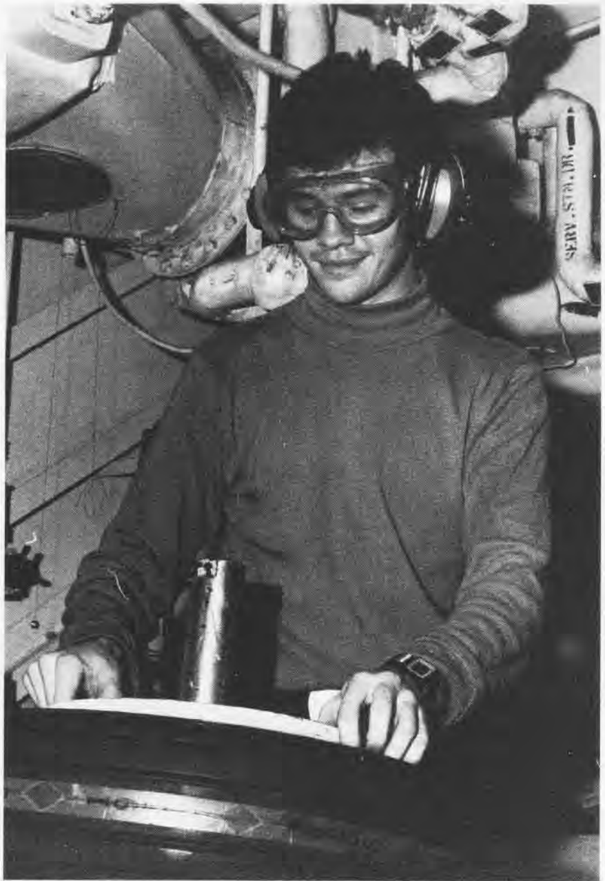
In the Theodore Roosevelt tire shop, AMSAR Brian Ward puts split rims together on an F-14 nose tire.
