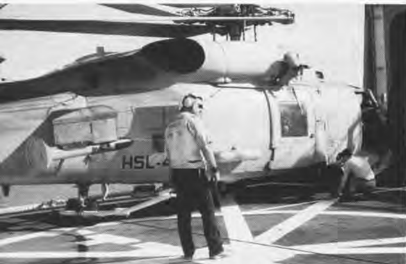
Robert Brennan, NAWC AD Lakehurst, observes cable alignment of the new SH-60B traversing system on George Phillip (FFG 12).
