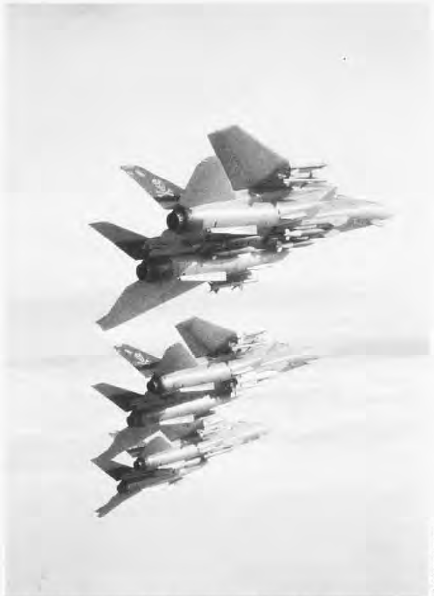
Three VF-84 F-14As carry external stores that exhibit the three missions of the Tomcat: (top to bottom) strike, interceptor, reconnaissance.
