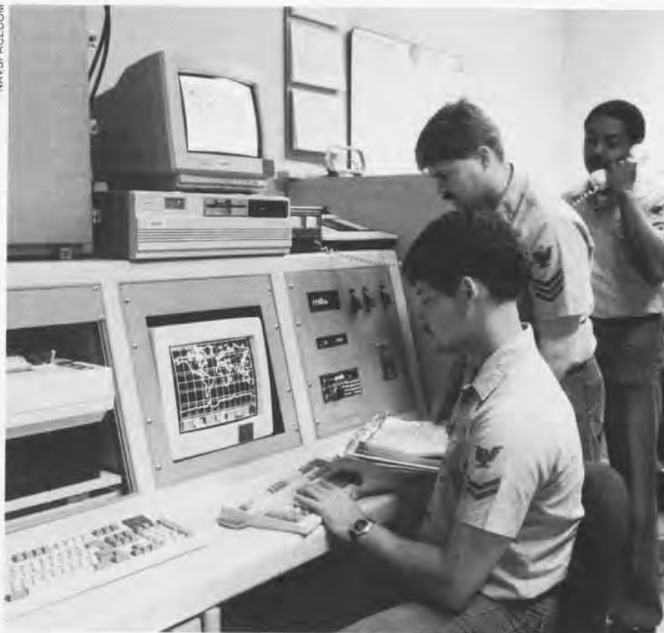
Naval Space Operations Center watchstanders at Dahlgren, Va., monitor the ground station for the Multiple-Access Communications Satellite, developed to provide store-and-forward communications for tactical commanders.
