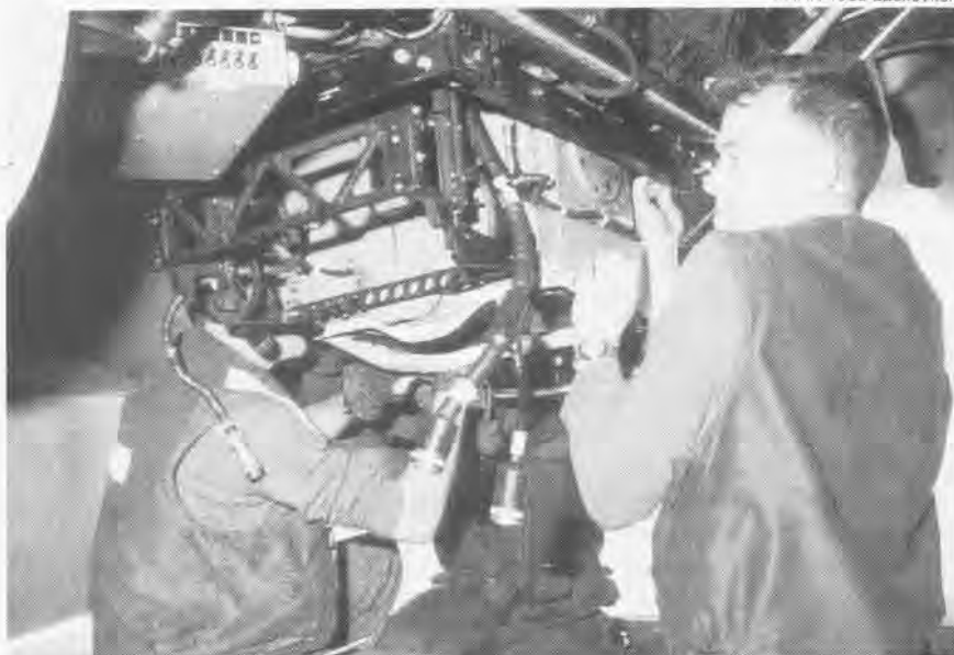
Two PHs remove an infrared sensor from a Tactical Air Reconnaissance Pod System (TARPS) pod on a VF-84 F-14A aboard Theodore Roosevelt (CVN 71) during Operation Deny Flight.
