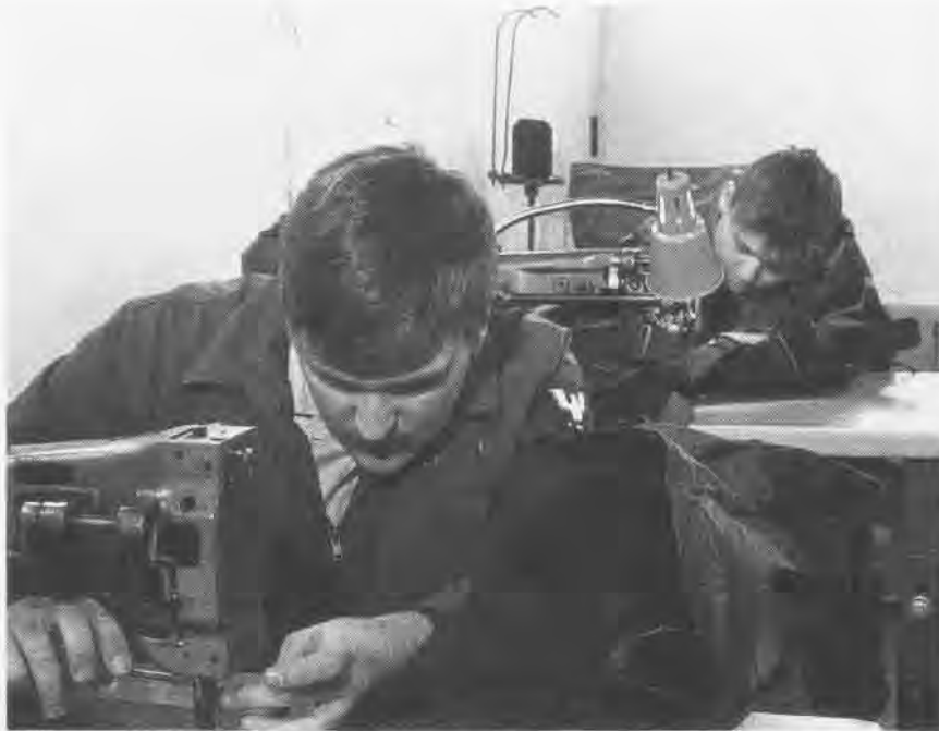
An important tool in any PR shop is the sewing machine, which is used for repairs on equipment and parachutes.
