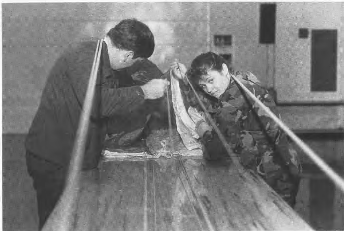
Checking to make sure all lines are straight, PR3 Mark Kilmer and Marine Sgt. Pamela Schaub demonstrate the proper method of packing a parachute.
