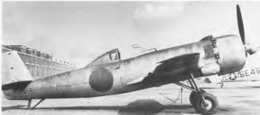
Although 105 Nakajima Ki.115 Tsurugi (Sabre) dedicated suicide planes were built, none were used operationally. The aircraft's main gear was jettisoned after takeoff, and the Tsurugi could carry a 1,764-lb. bomb.
