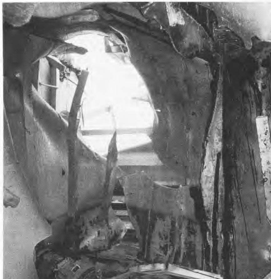
The Harpoon impact caused this hull damage to the patrol craft target.
