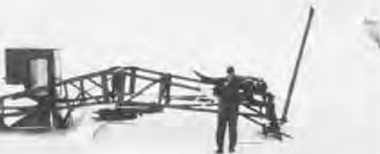
LCdr. Hinebaugh explained that snow planes like this one are dragged by tractors to prepare skiways at established camps which have regularly scheduled flights.
