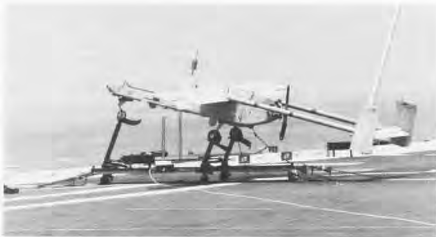
Rocket assisted launchers such as this one aboard Denver (LPD 9) allow Pioneers to launch from virtually anywhere.
