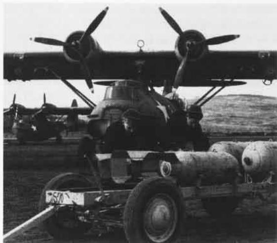
The Navy initially experimented with gun turrets on several types of aircraft, including patrol planes such as this PBM Mariner. Turrets were removed from early production Mariners because of weight problems, but installed in all later models.
