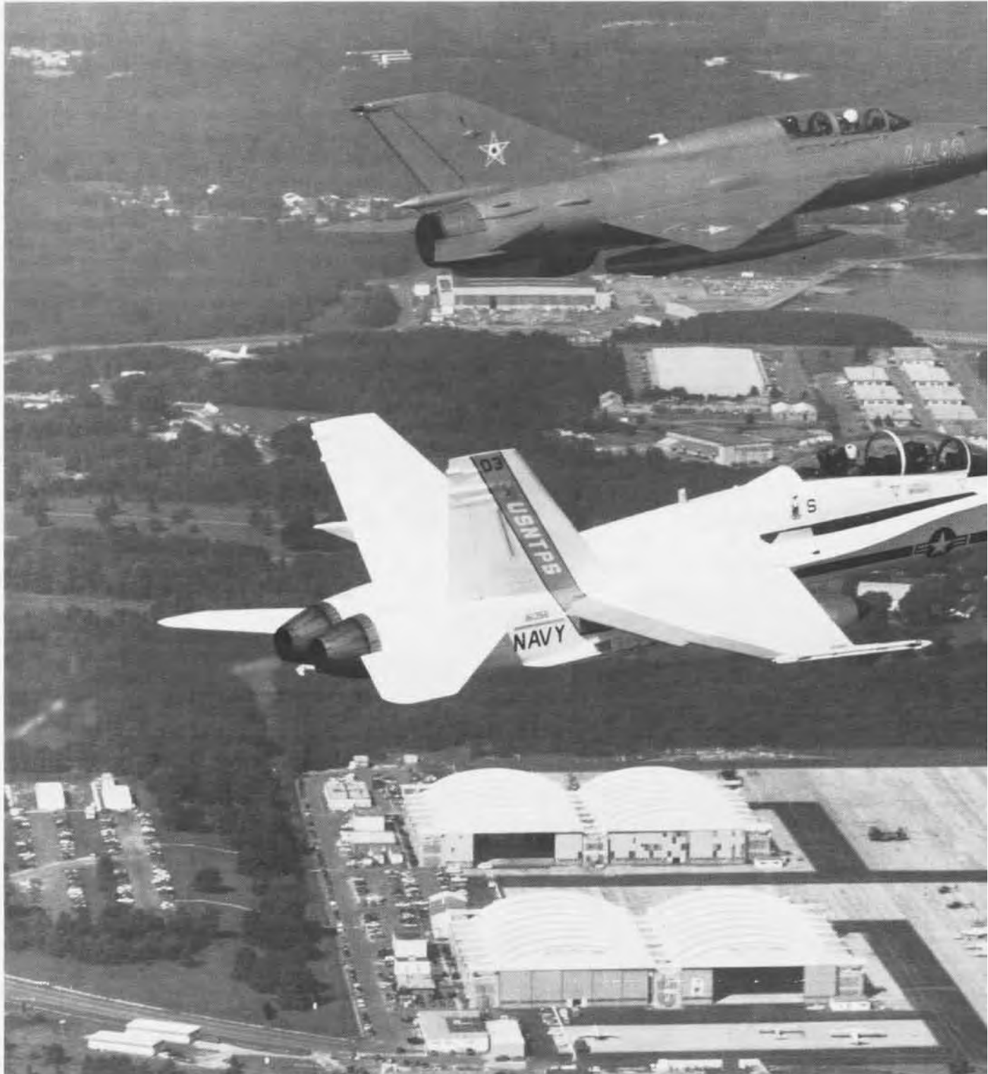
A TF/A-18 Hornet, the newest airplane in the U.S. Naval Test Pilot School inventory, makes a pass over the school ramp and hangar area accompanied by a Russian MiG-21U, which is occasionally contracted to the school for training purposes.
