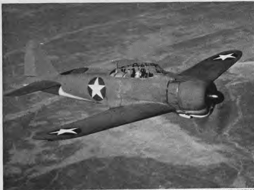
ZEKE IS KNOWN FOR ITS LOW WING LOADING, STEEP ANGLE OF CLIMB AND STURDY CONSTRUCTION
