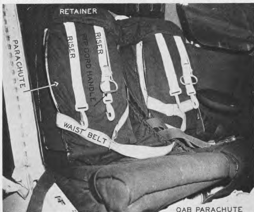
QAB PARACHUTE FORMS BACK CUSHION OF SEAT; RISERS AND BELT READY FOR EASY ATTACHMENT
