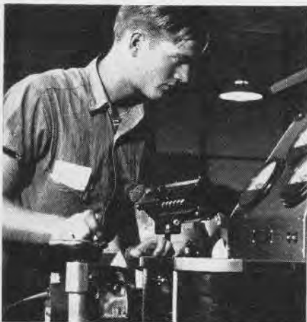
CHECKING the magneto on a test bench to see if its speed, output, and sparking gap are adjusted for maximum power output required by an airplane's engine.
