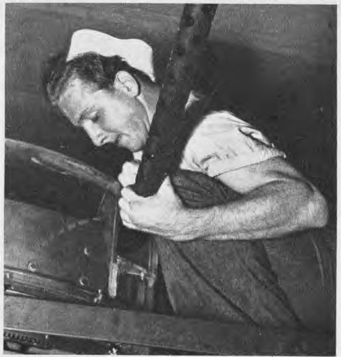
AN AVIATION ordnanceman installing a .50 caliber machine gun in a power-operated deck turret on one of the Navy's fighting planes. Without its guns operating in tiptop shape the plane can be expected to do very little more than run.
