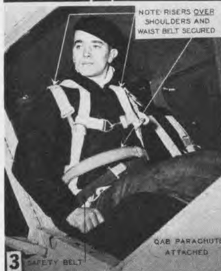
BUREAU REVEALS CORRECT METHOD OF DONNING QUICK ATTACHABLE BACK PARACHUTE FOR FLIERS
