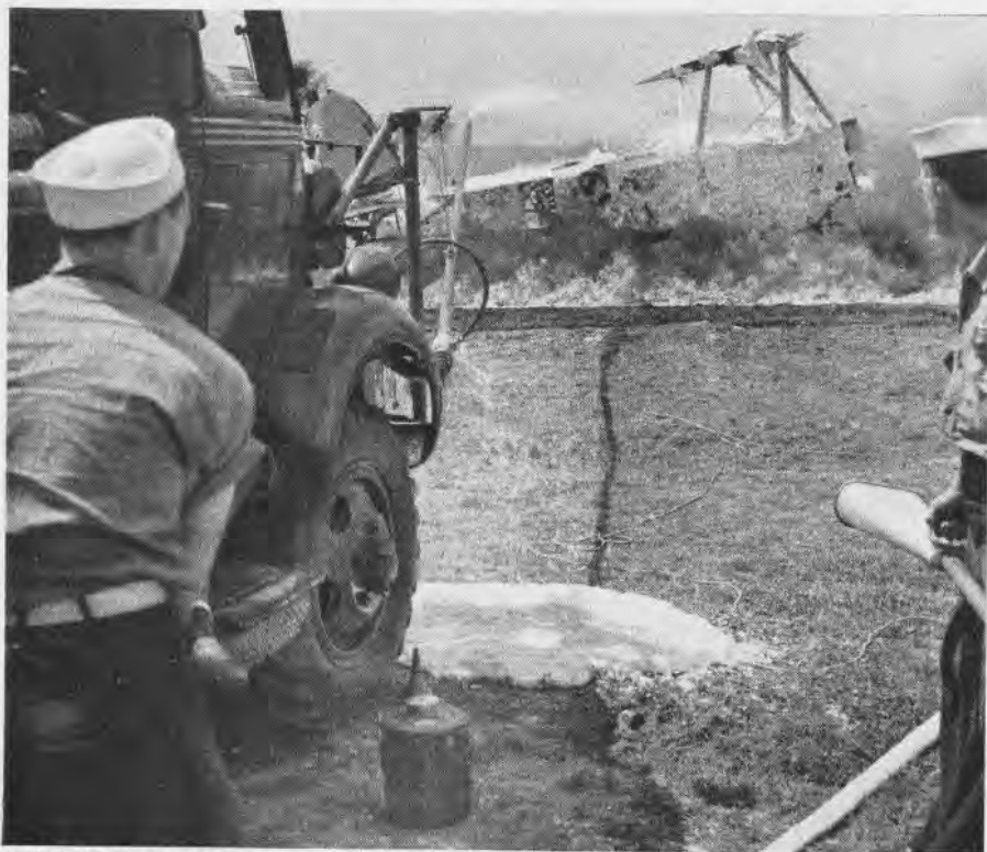
FOAM SWIVEL BOOM ATTACHED TO TRUCK SPEEDS RESCUE OF NAVAL AVIATORS CAUGHT IN WRECKAGE
