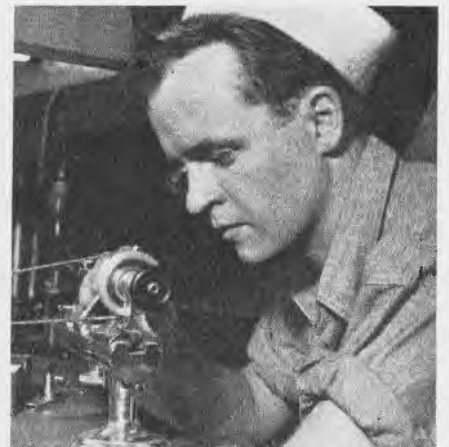
EVEN FORMER WATCHMAKERS, like this one, find a place for their talents polishing up electrode tips on sparkplugs, using jeweler's lathe as well as magnifier.
