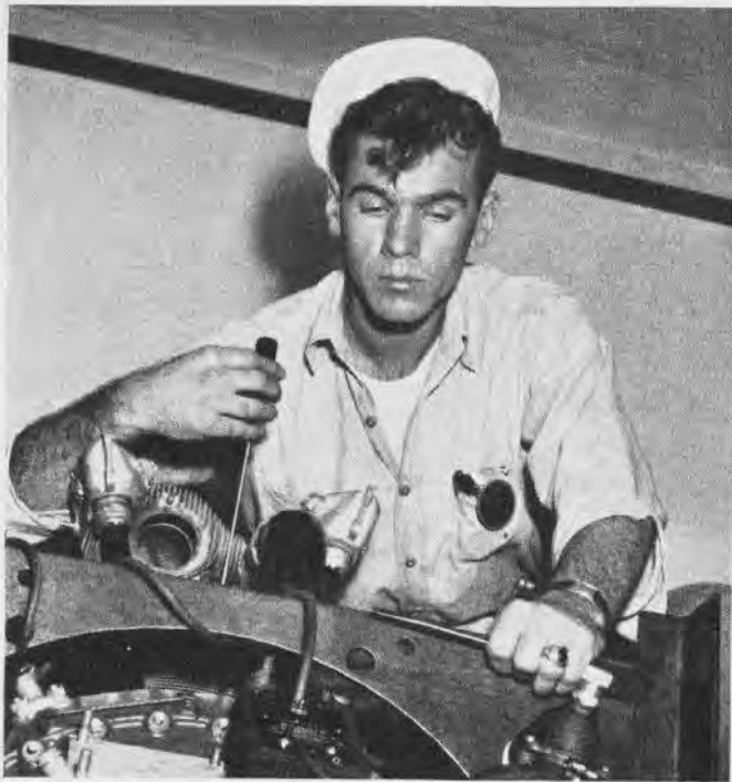
SYNCHRONIZED TIMING of an airplane engine's two magnetos is necessary if its cylinders are to fire correctly. Using a timing light device in the synchronization process greatly simplifies the delicate operation for this aviation machinist's mate.
