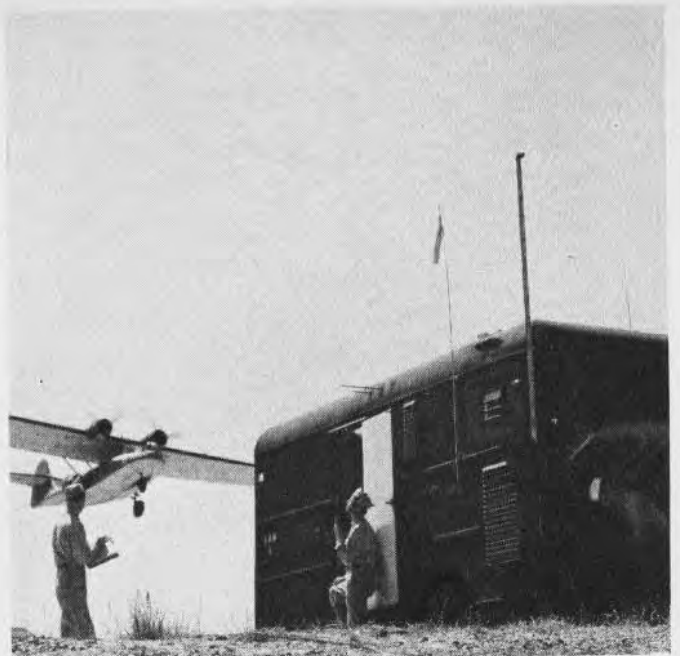
YB-ZA RADIO MARKER INFORMS PBY PILOT THAT HE IS OVER RUNWAY EXPERIMENTAL YB-ZA EQUIPMENT TRANSMITS CURVED BEAM FOR LANDINGS
