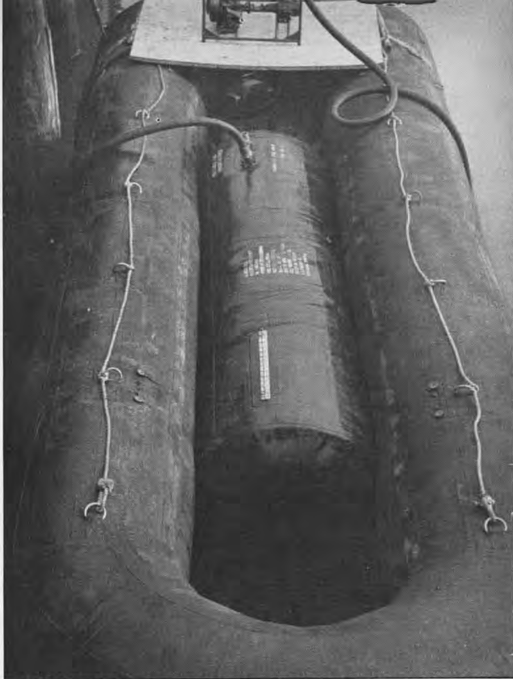
TWO RUBBER PLANE-REFUELING CELLS, THE 550-GAL. (ABOVE) AND THE 2,000-GAL. TYPE (BELOW)
