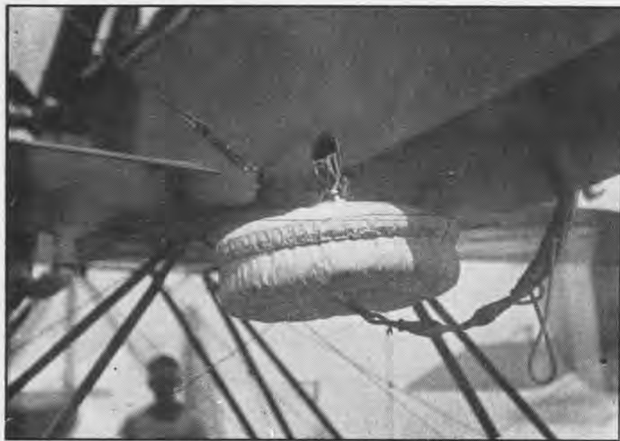
NAVAL SEAPLANE USED DURING FIRST WORLD WAR WITH PARACHUTE ATTACHED TO FUSELAGE
