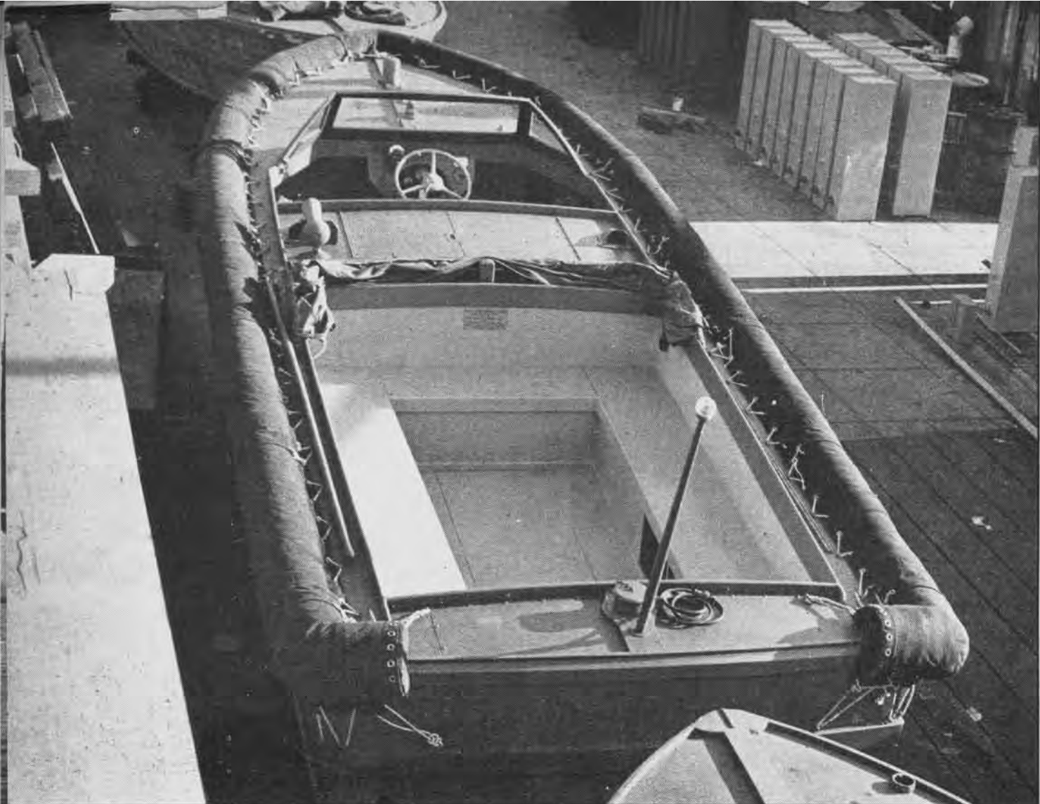
NAVY'S NEW PERSONNEL BOAT USED TO TRANSPORT CREWS TO AND FROM SEAPLANES; CRAFT HAS 25-KNOT SPEED TO GET TO INSHORE CRASHES
