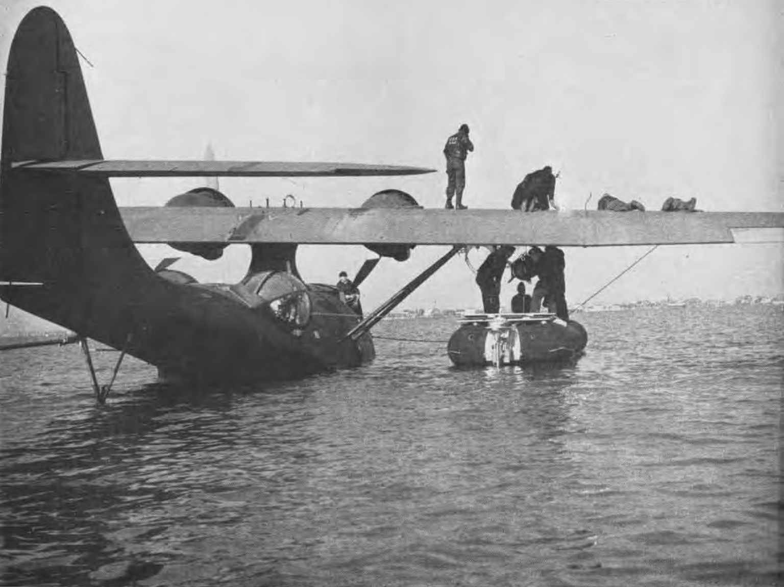
RUBBER REARMING BOAT, FITTED WITH OUTBOARD MOTOR, USED TO LOAD BOMB ON SEAPLANE RACK. LARGEST OF TYPE ARE AMMUNITION LIGHTERS
