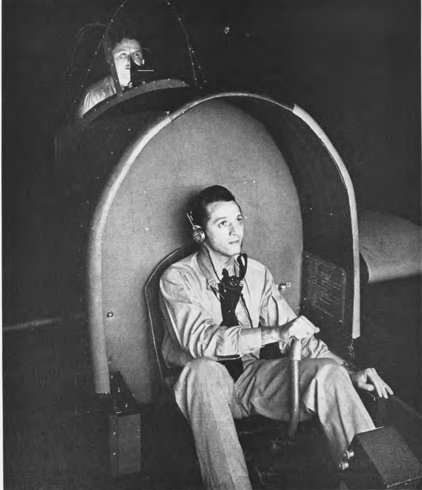
GUNAIRSTRUCTOR IS A TWO-MAN MECHANISM IN WHICH THE INSTRUCTOR ATTEMPTS TO OUTWIT HIS STUDENT BY MANEUVERING TARGET ON SCREEN
