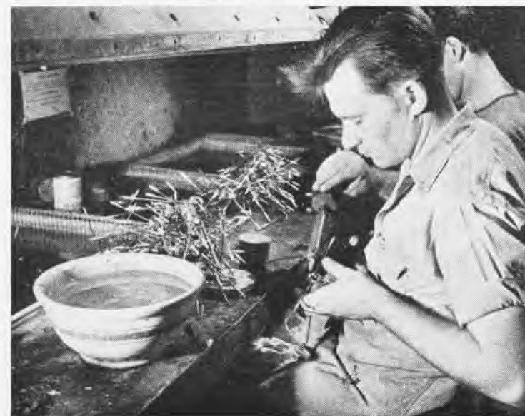
WORKERS GIVE STRICT ATTENTION TO ASSEMBLY OF PILOT CHUTE FRAMES
