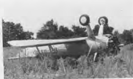
THIS IS WHAT OFTEN HAPPENS WHEN SIMULATED EMERGENCY LANDINGS ARE CARRIED BELOW PRESCRIBED ALTITUDE.
