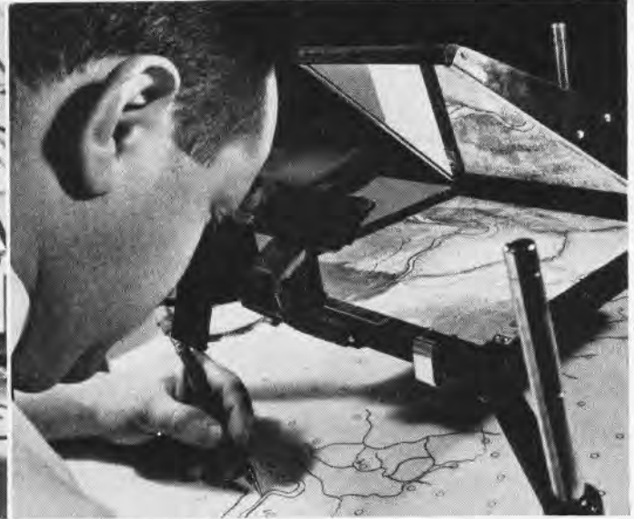
12 SKETCHMASTER projects negative on paper where it is traced to form scaled map of enemy territory
