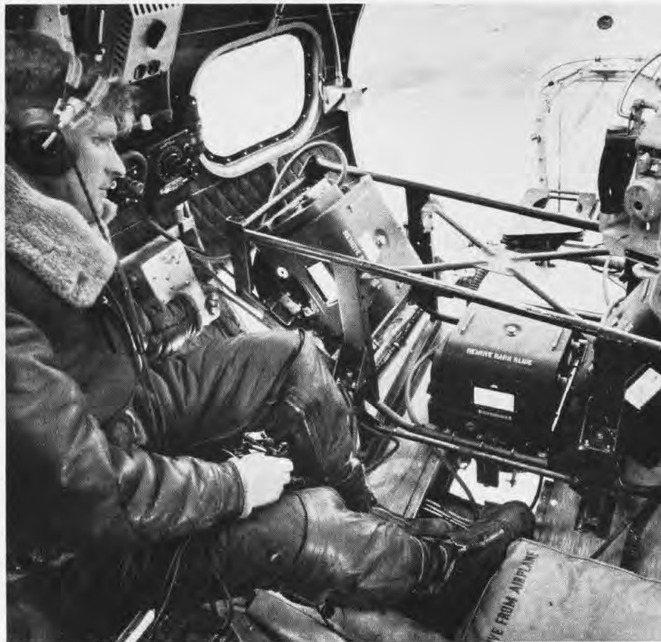
CAMERA IN CENTER SHOOTS VERTICALLY DOWN. THOSE ON SIDES OBLIQUELY TO HORIZONS
