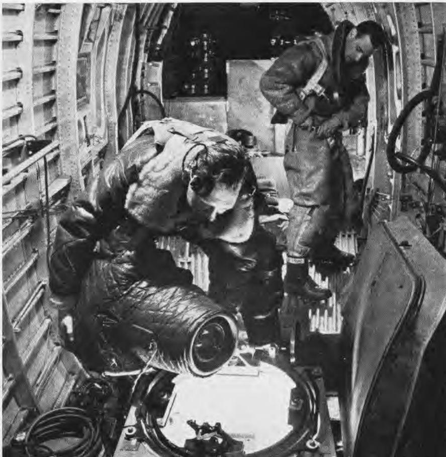
SNUG JACKETS KEEP ELECTRICALLY HEATED CAMERAS IN 'GOOD CONDITION AT HIGH ALTITUDES
