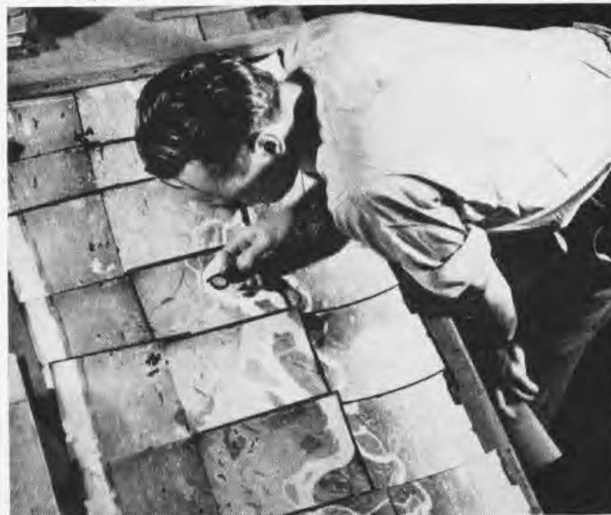
13 MOSAICS prepared by matching overlapped prints in long strips give the complete picture of area
