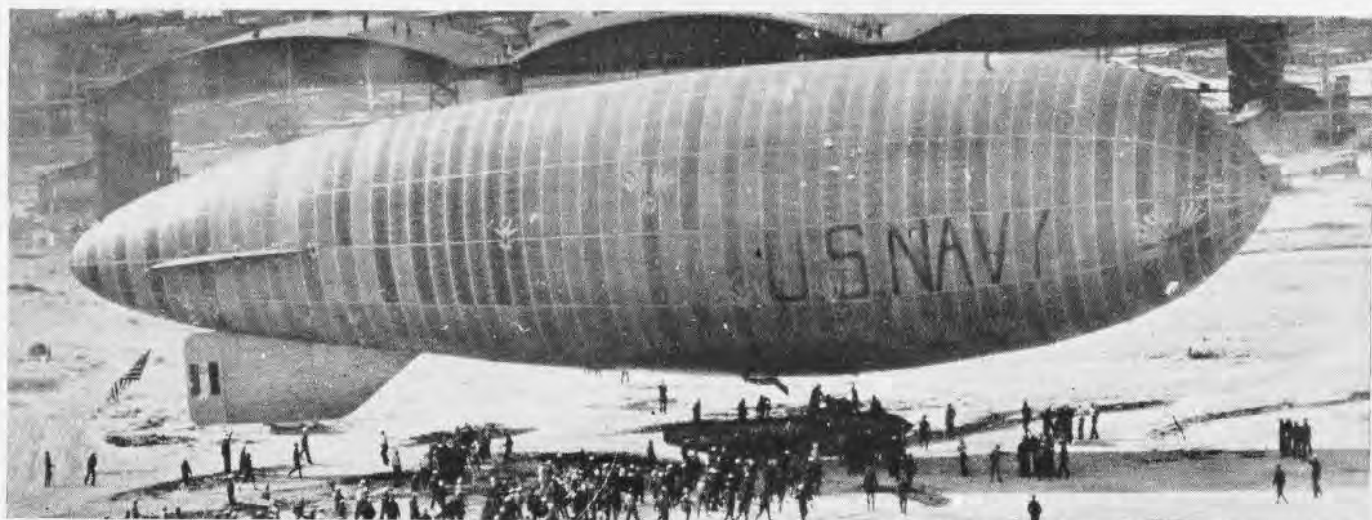
NON-RIGID AIRSHIP C-1 DEVELOPING SPEEDS UP TO 60 MPH FROM TWIN 150 HORSEPOWER ENGINES IS TEST FLOWN FROM AKRON TO ROCKAWAY, L. I.
