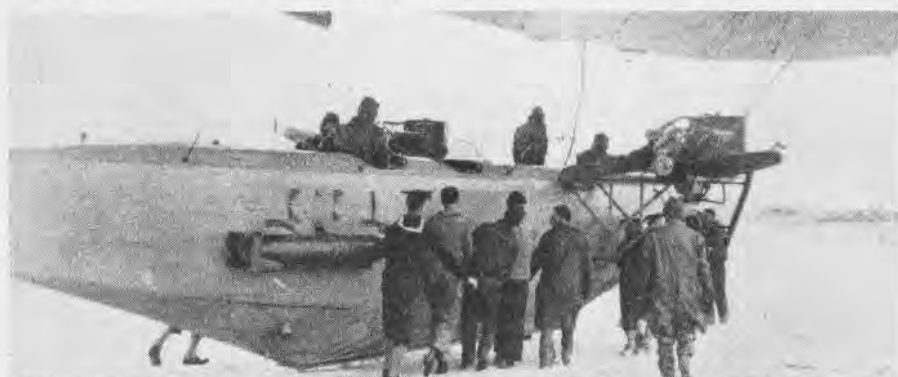
FIRST “C” TYPE NONRIGID DIRIGIBLES, COMPLETED IN SEPTEMBER 1918, HAD SPEED OF 60 MPH
