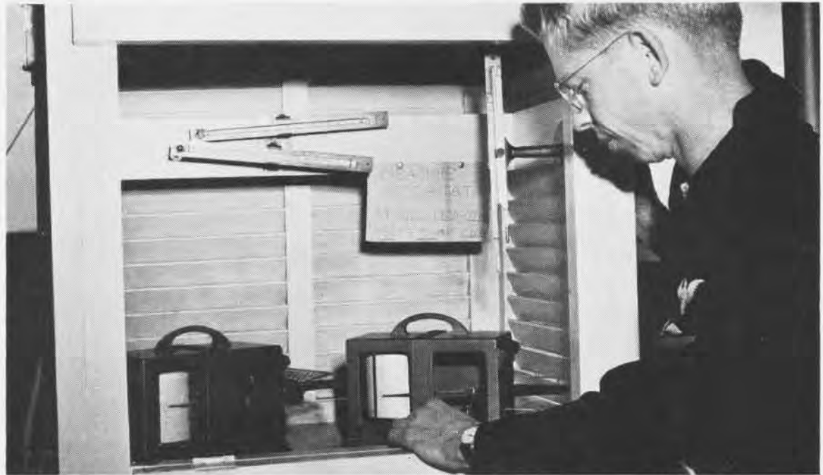
2 THERMOGRAPH records temperature weekly. To left is humidity-recording hydrograph. Maximum & minimum thermometers are on wall. Psychrometer, used to obtain wet & dry bulb temperatures, is on rotor at right
