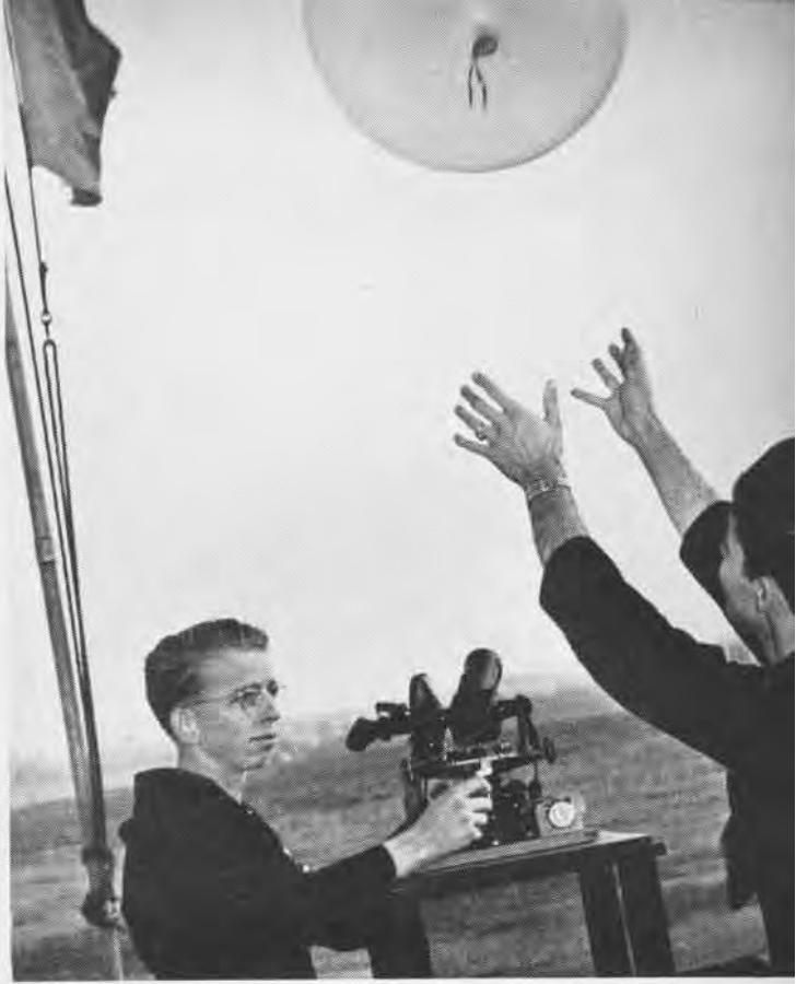
5 PILOT balloon is released to check winds aloft. Then theodolite measures elevation and azimuth angle of balloon in air
