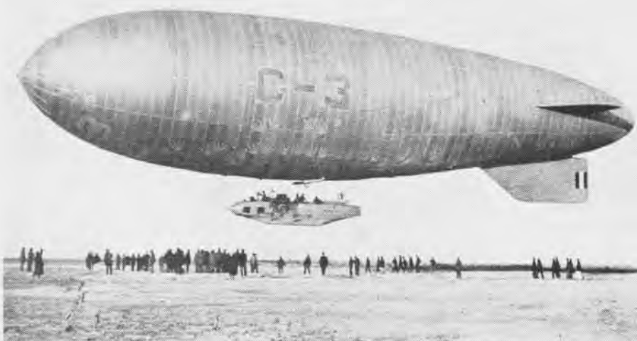
C-TYPE AIRSHIPS WERE DESIGNED IN 1918 TO CARRY DEPTH CHARGES FOR ANTI-SUB ACTIVITIES
