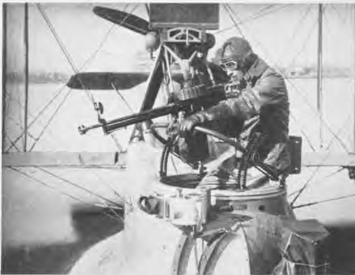
PILOT had to stand up to operate Lewis machine gun on seaplane; today cockpit armor offers great protection to plane occupants
