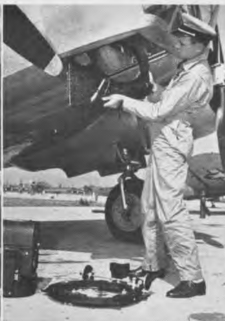
MOUNT INSTALLS IN PLACE OF ESCAPE HATCH
