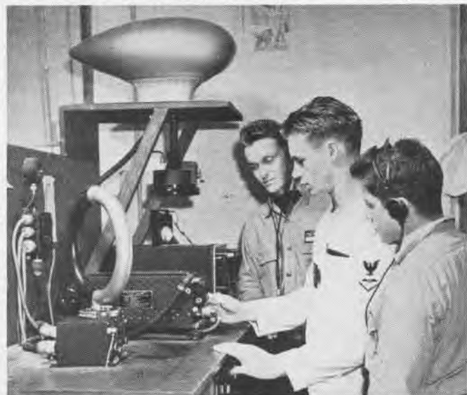
OPERATION of DU and DZ homing devices are introduced during aviation radiomen's training, must be thoroughly mastered
