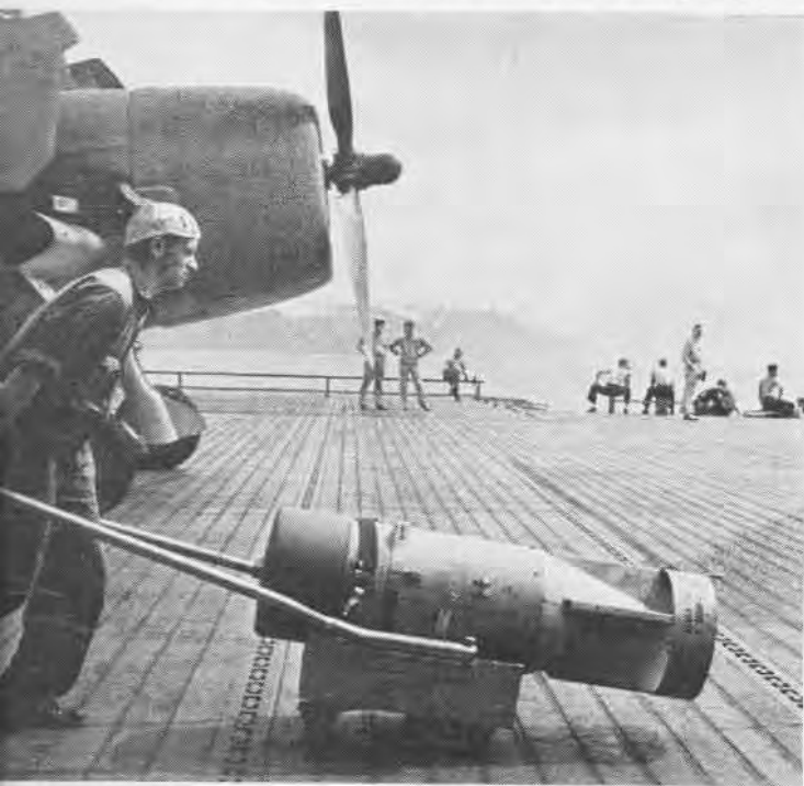
ORDNANCE Bureau furnishes both depth bomb and bomb skid which ordnanceman is trundling on carrier deck past Hellcat
