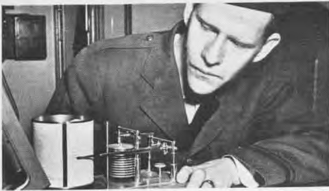
3 LAMBERT FIELD aerology officer carefully checks barograph which gives continuous weekly record of barometric pressure
