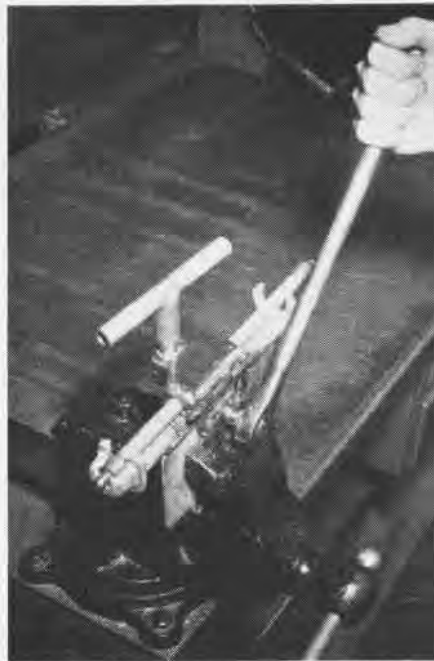
JIG ELIMINATES DAMAGE TO ROD BALL ENDS
