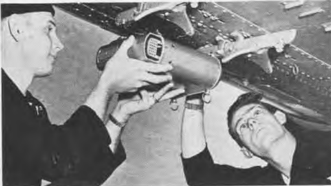
4 AEROGRAPH records pressure, temperature, and humidity to height of about 3 miles when carried aloft by service aircraft
