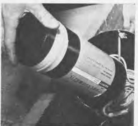
BUNGEE TENSION EJECTS CAN WHEN RELEASED
