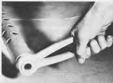
WRENCH FACILITATES TURNING OF GUN BARREL
