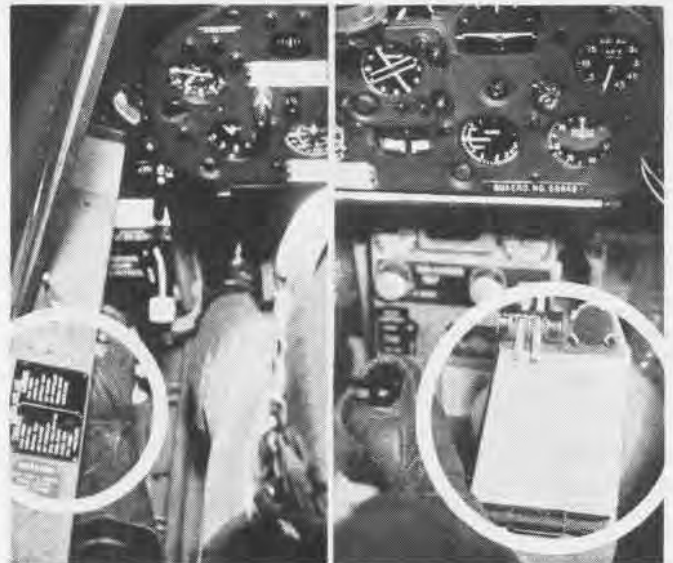
Use of check-off list is just as important to the ferry pilot as any other naval aviator; on left is the list attached to the plane, at right is the check-off pad fastened to pilot's knee for convenience
