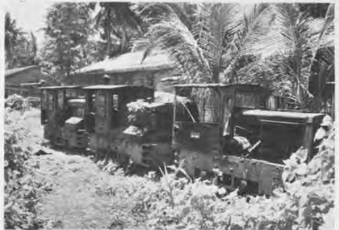
Gasoline-powered locomotives operated on the narrow gauge track running from the warehouses to end of pier, possibly to fuel dump
