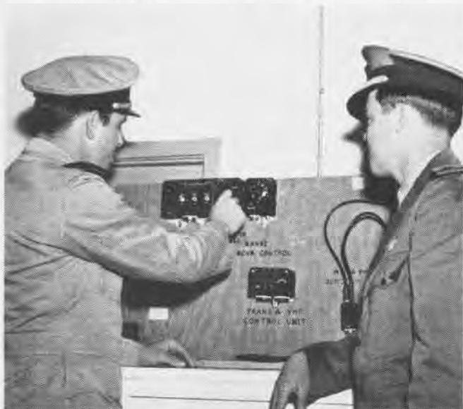
Mockup board of radio installations is used to check out men, to be sure they know how to use the type installed in plane they will be ferrying; "green" pilots usually "know" the most
