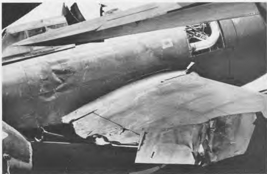
THIS COMBAT PLANE TOOK A TERRIFIC BEATING IN HIGH WINDS ENCOUNTERED BY ESCORT CARRIER
