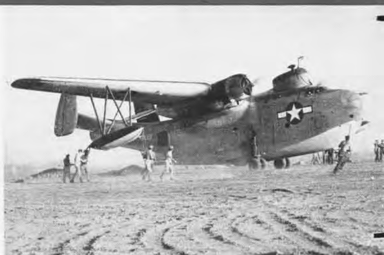
DOUBLE-TIRED WHEELS WERE ATTACHED ON REINFORCED MOUNTS
