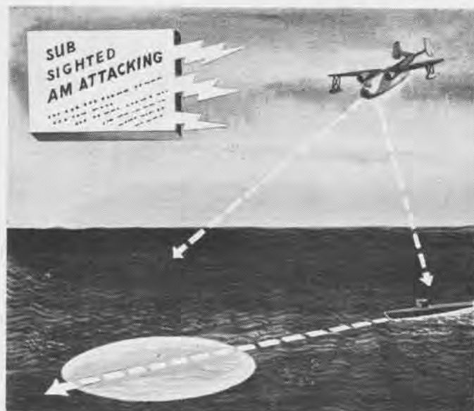
1. Sub sighted and normal surface attack is planned. Sub (200 ft.); speed 17 knots (28 ft. per second); intervalometer set for six-bomb stick, 60 ft. spacing. Pilot projects the aiming circle
