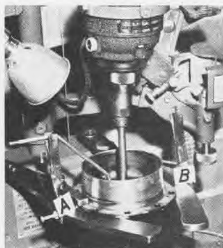
CLIPS SIMPLIFY WORK ON GRINDING MACHINE
