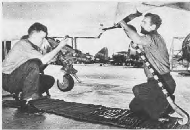
Installation of tail wheel and arresting gear assembly comes under Structures; Hydraulics, Power Plants, Operation also are studied
