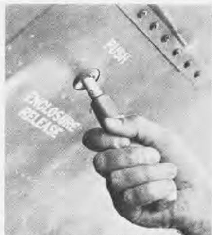
SIMPLE RELEASE TOOL HELPS OPEN PLANE HOOD
