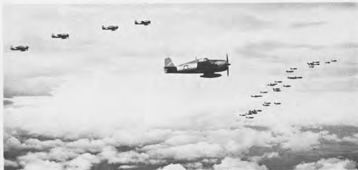
F6F HELLCAT FIGHTERS CARRYING EXTRA FUEL IN BELLY TANKS ESCORT AVENGER TORPEDO BOMBERS AND DAUNTLESS DIVE BOMBERS ON A STRIKE
