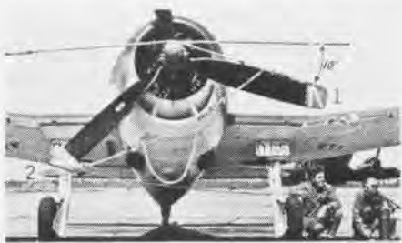
PULL ENGINES THROUGH WITH BUNGEE STARTER
