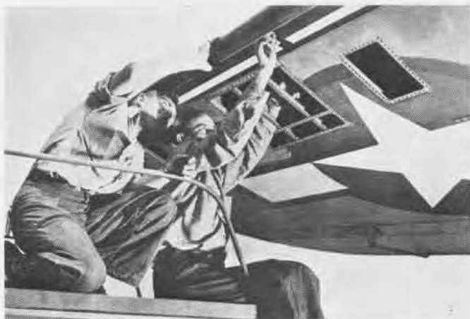
Training in line maintenance covers all the structural aspects of the plane. Students above adjust wing slats, one of many jobs
