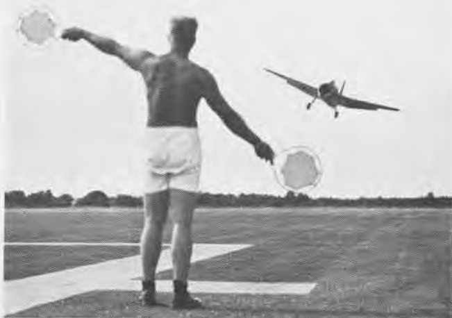
Landing signal officer guides student in field carrier landing. Pilot learns carrier technique before qualifications at sea
