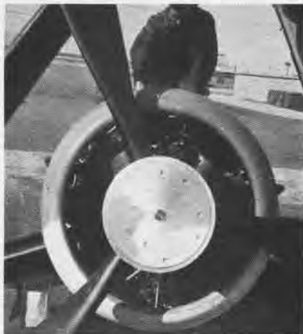
DISC REVEALS WHEN VALVES NEED ADJUSTING
