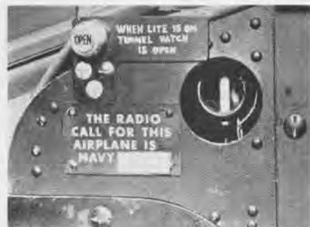
RED LIGHT SHINES IF HATCH IS NOT CLOSED
