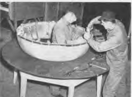
CIRCULAR BENCH AIDS WORK ON RING COWLINGS
