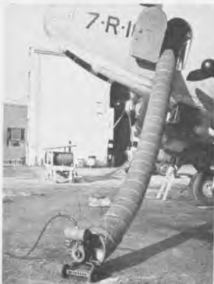
VENTILATOR BLOWS AIR TO COOL HOT AIRCRAFT
