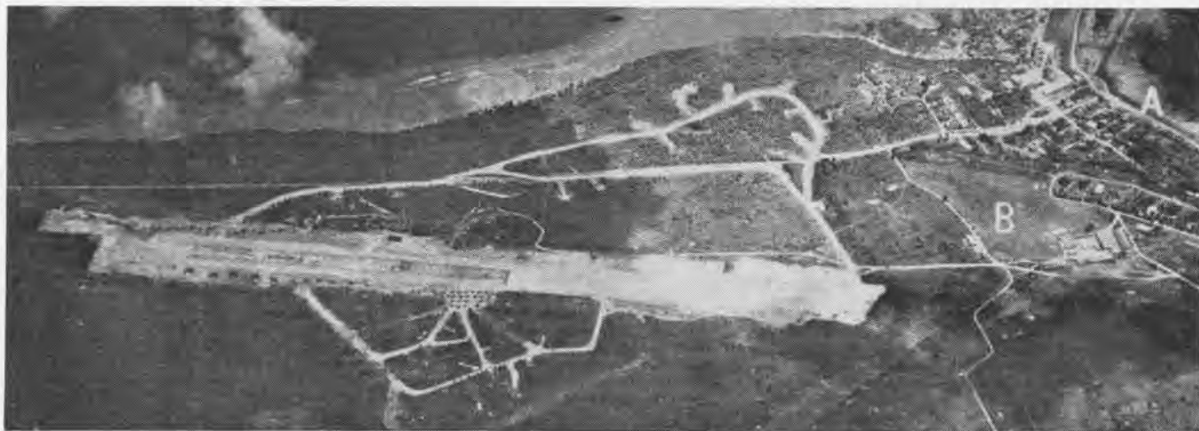
Photo reconnaissance by a Navy plane before the assault on Guam island revealed this important airfield on Orote Peninsula near Sumay. Runway is 320' x 5,400'. Of this area, 140' x 2,240' is paved, the rest has crushed coral surface. Strip bristles with Jap planes
