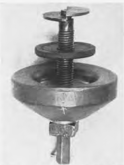
TOOL FORCES SHEET METAL AGAINST THE DIE
