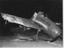
sharply to the right and nosed up. The fuselage broke aft of the cockpit.
