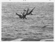
As soon as the plane became airborne, the wing continued folding and was torn off. The *Corsair* rolled to the left and hit the water off the port bow of the ship in a 35° nose down, inverted position. The plane sank immediately with the pilot apparently unable to get clear.
